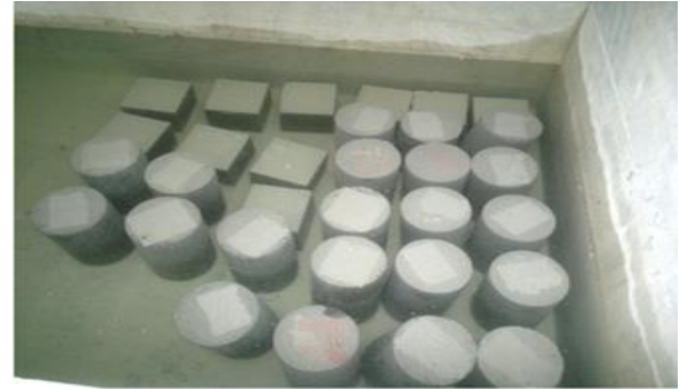
Fig. 1 The specimens were taken out of the molds and kept for 26 days in a pool
