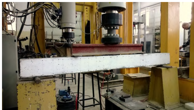
Fig. 1 Test set-up, beam located under hydraulic jack and prepared for measurement
