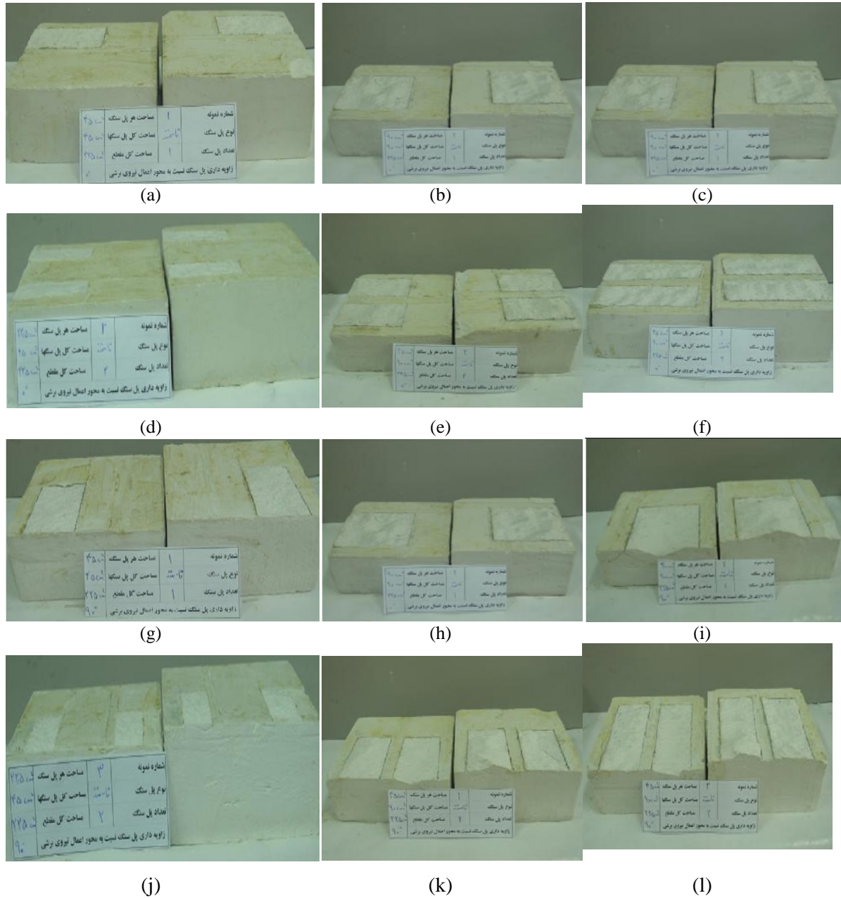
Fig. 6 The failure patterns in non-persistent rock bridges
