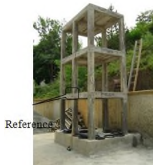
Fig. 5 A typical measurement setup with reference signal
