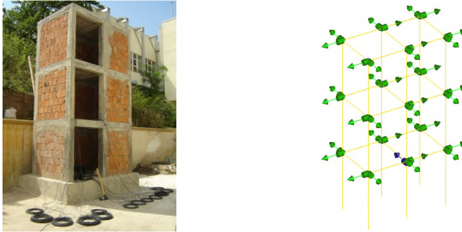
Fig. 15 The measurement on the brick-walled building model
