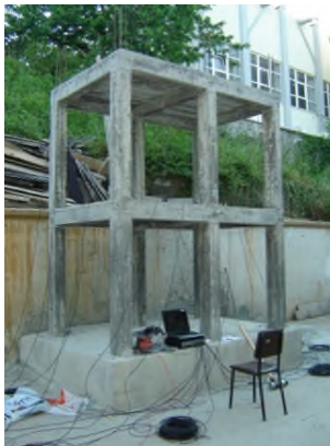
Fig. 9 The measurement setup on the two-storey building model
