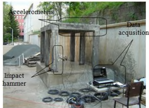
Fig. 3 A typical measurement setup on the RC building model
