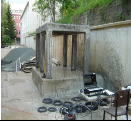
Fig. 6 The measurement setup on the one-storey building model
