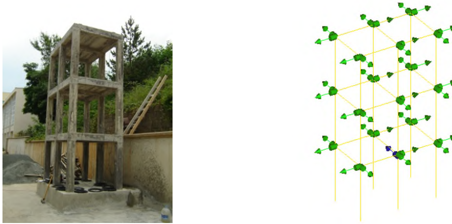
Fig. 12 The measurement setup on the three-storey building model
