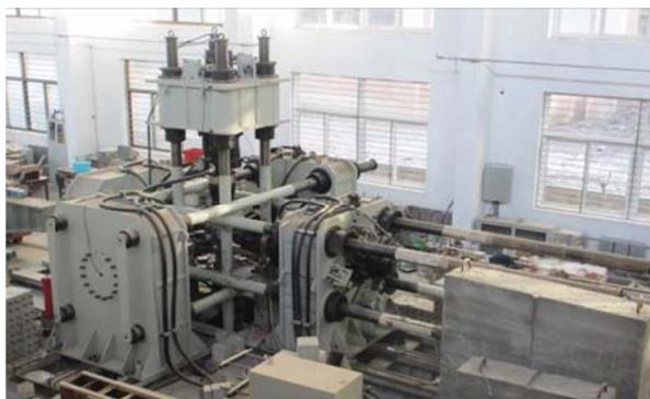
(a) the triaxial testing machine
