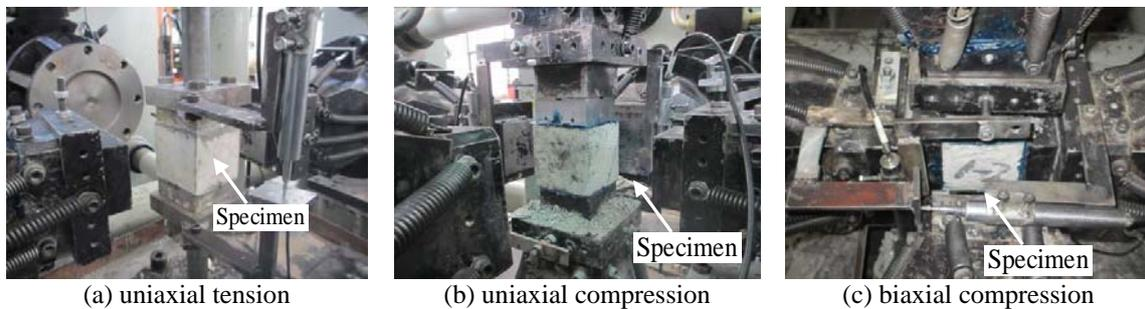
Fig. 3 States of the specimen in triaxial testing machine
