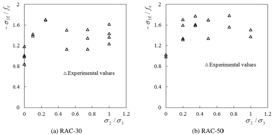
Fig. 5 The influence of the stress ratios on the principal stress  $-\sigma_{3f}/f_c$  under biaxial compression
