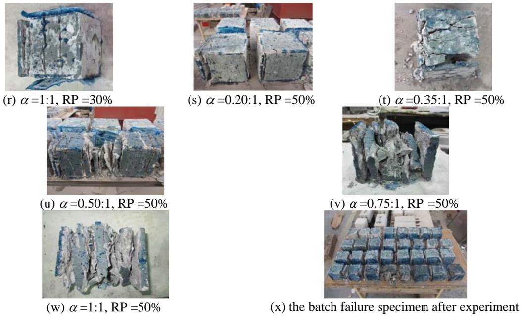
Fig. 4 Failure modes of plain RAC under multiaxial stress states
