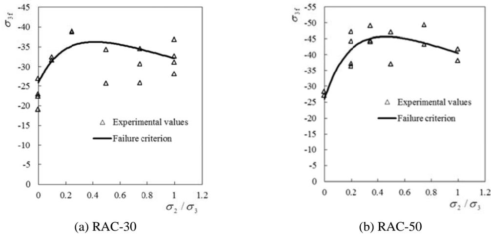
Fig. 6 The comparison of Eq. (1) and test values under biaxial compression
