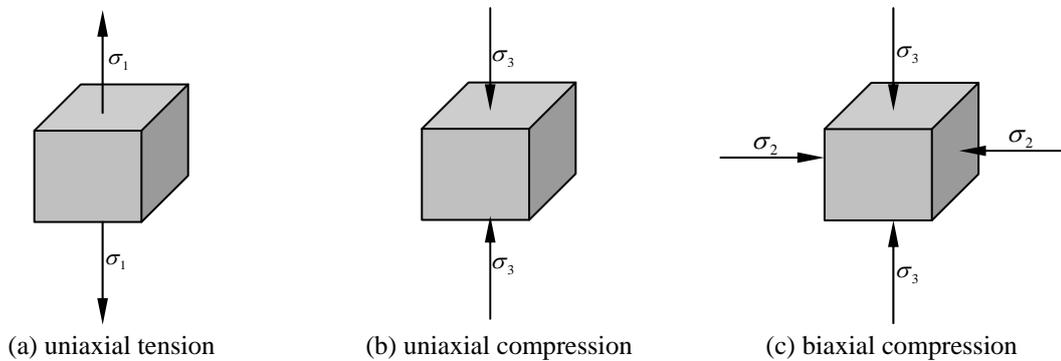
Fig. 2 Uniaxial and biaxial loading directions
