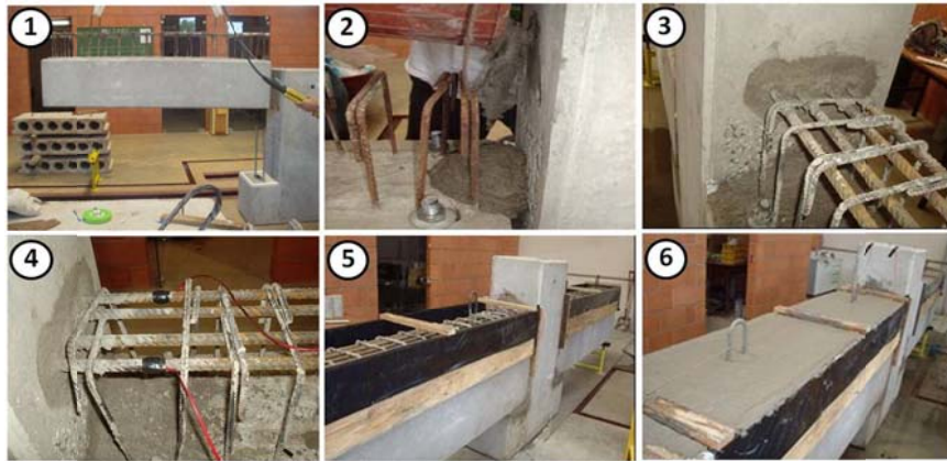
Fig. 3 The assembly sequence of experimental model
