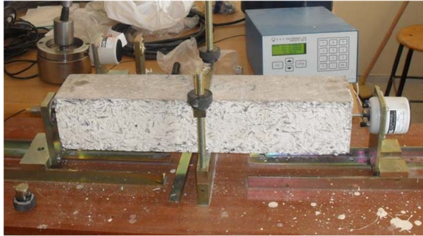
Fig. 2 Resonance frequency measurement on concrete
