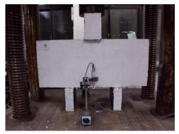
Fig. 2 Testing arrangements for deep beams
