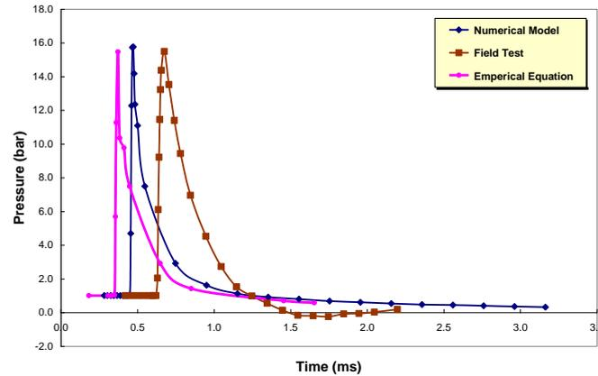
Fig. 13 Pressure-time history hitting the centre of the RC panel using 2-kg TNT explosive
