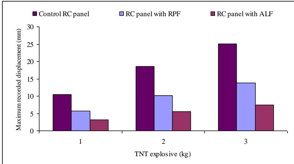
Fig. 16 Maximum recorded displacement at the centre of RC panel strengthened by the RPF and the ALF layer under different TNT explosives
