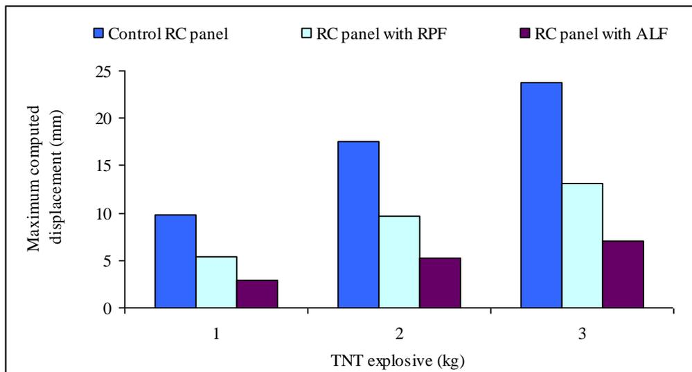
Fig. 15 Maximum computed displacement at the centre of RC panel strengthened by the RPF and the ALF layer under different TNT explosives
