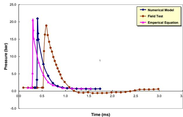
Fig. 14 Pressure-time history hitting the centre of the RC panel using 3-kg TNT explosive
