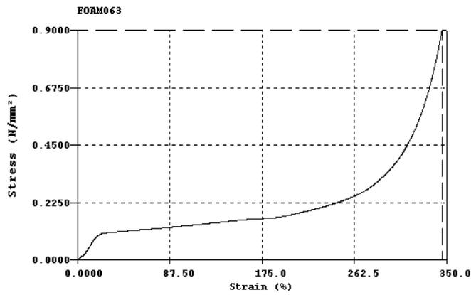
Fig. 9 Stress-strain curve of the aluminium foam (ALF)
