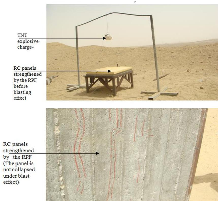
Fig. 18 RC panel strengthened by the RPF layer subjected to 3-kg TNT explosive charge
