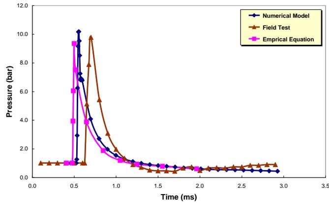
Fig. 12 Pressure-time history hitting the centre of the RC panel using 1-kg TNT explosive
