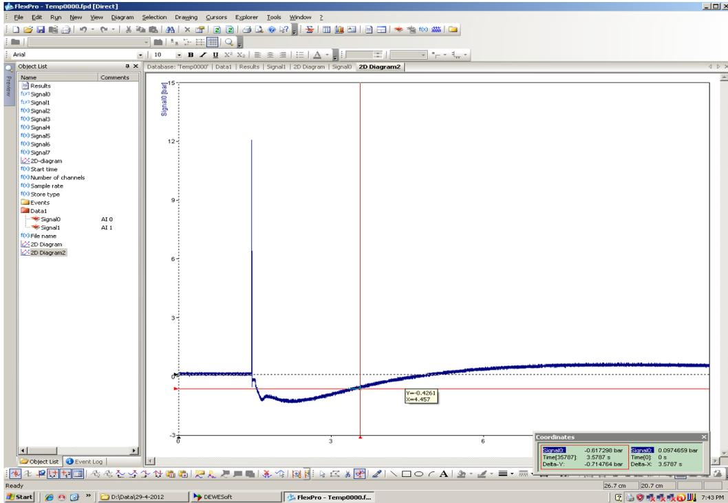
Fig. 5: Recorded pressure-time history hitting the RC panels using 2 kg-TNT explosive
