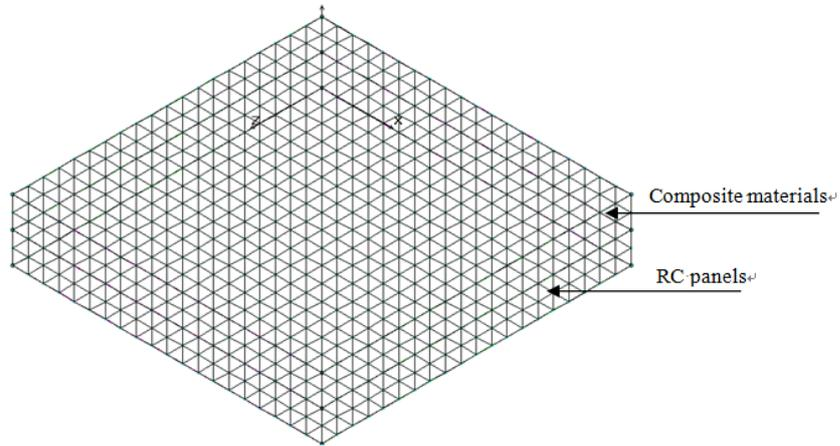
Fig. 7 3-D finite element model of the RC panels strengthened by composite materials
