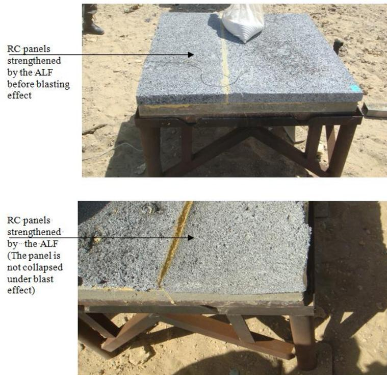
Fig. 19 RC panel strengthened by the ALF layer subjected to 3-kg TNT explosive charge
