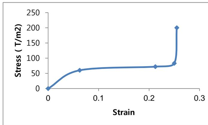
Fig. 8 Stress-strain curve of the rigid polyurethane foam (RPF)
