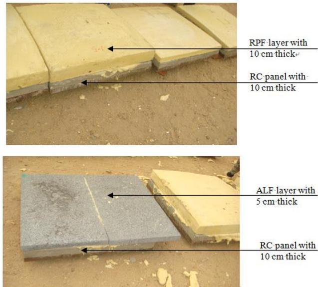
Fig. 2 Assembled reinforced concrete (RC) panels strengthened by the RPF and the ALF
