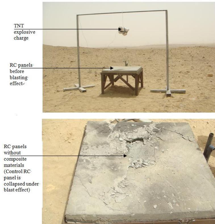
Fig. 17 Control RC panel subjected to 3-kg TNT explosive charge
