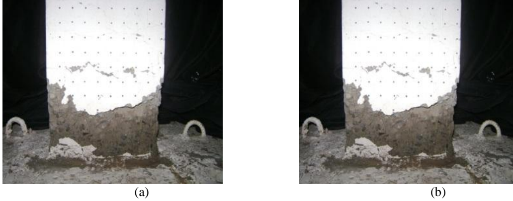
Fig. 7 Final damage observed in CRCS-60-32 column cast with 32 Mpa concrete (a) positive loading face (b) Negative loading face
