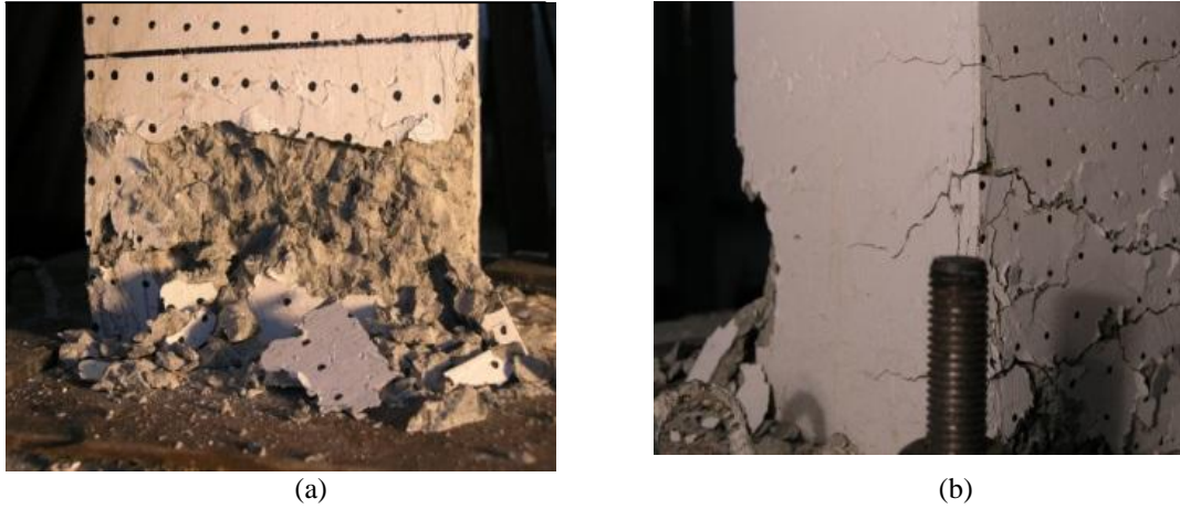
Fig. 5 Final damage observed in CRCS-60-25 column cast with 25 Mpa concrete (a) positive loading face (b) Negative loading face
