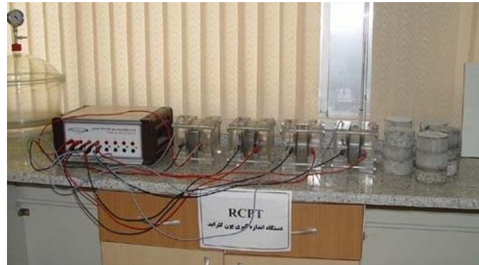
Fig. 4 The RCPT test set-up and apparatus used
