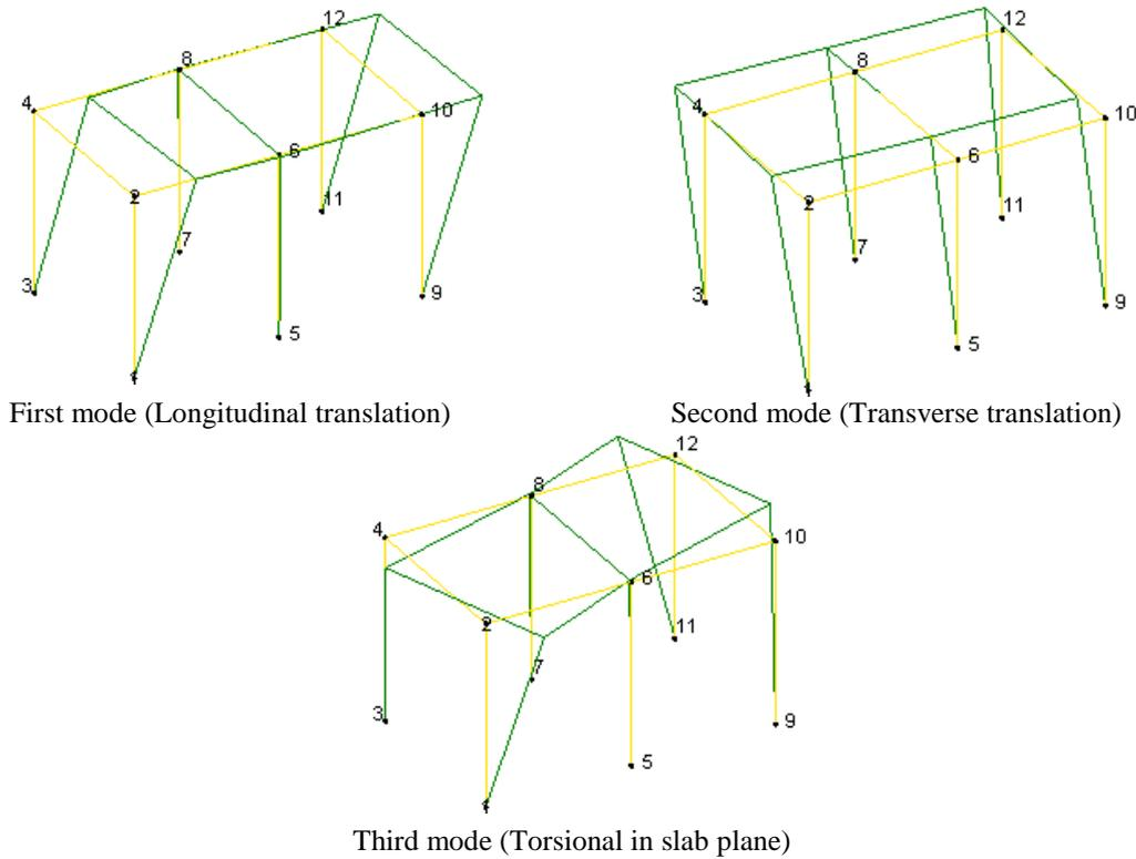
Fig. 9 The experimentally identified modal behaviors of the building model
