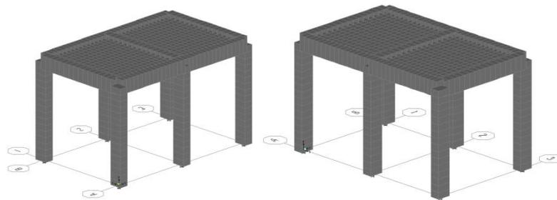
Fig. 3 The initial finite element model of the one storey reinforced concrete building model
