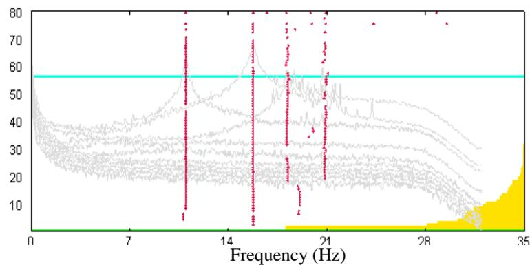
Fig. 14 The stabilization diagram for the second damage case of the building model
