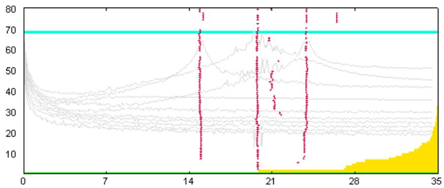
Fig. 7 The stabilization diagram for the undamaged building model
