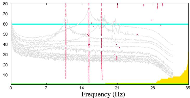
Fig. 16 The stabilization diagram for the third damage case of the building model
