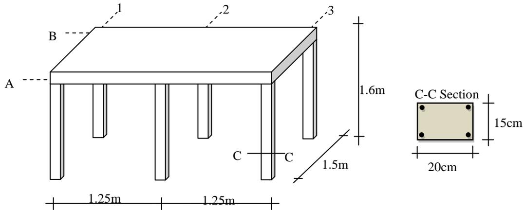
Fig. 1 The dimensions and sectional properties of the one storey building model
