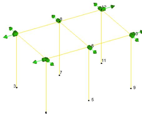
Fig. 5 The accelerometer directions and connections on the building model
