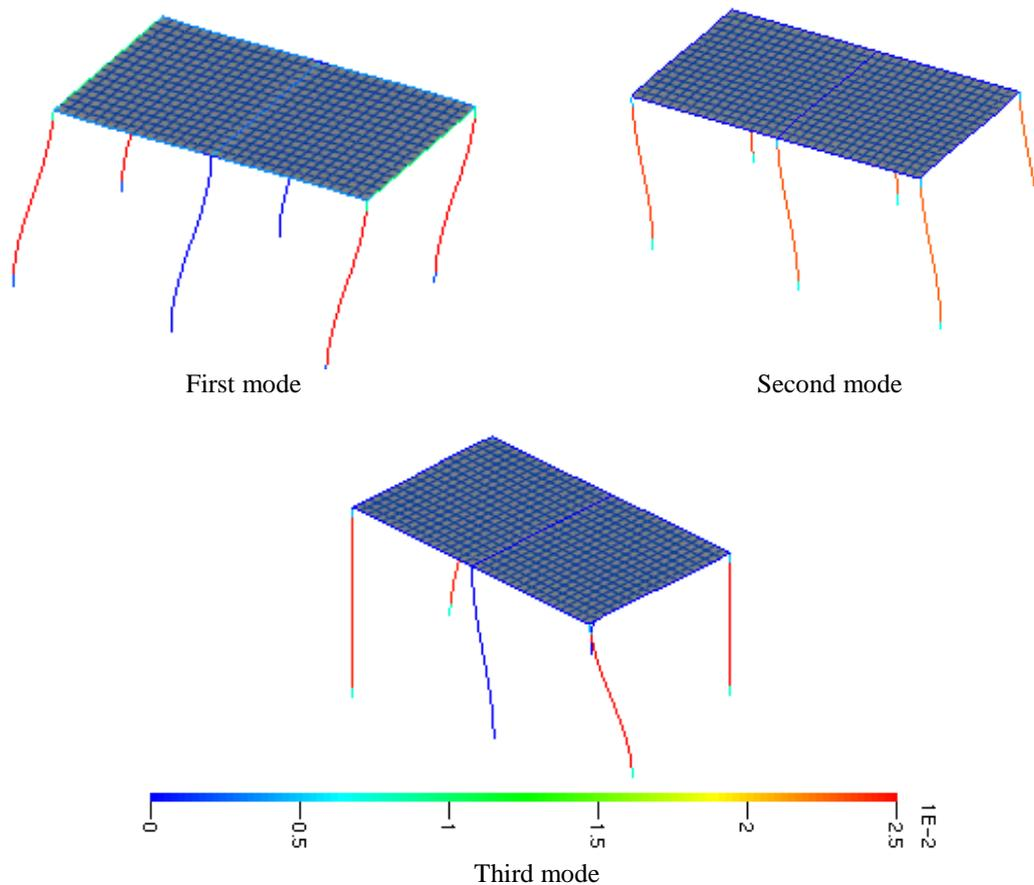
Fig. 17 The sensitivity analysis result on the first three mode shapes
