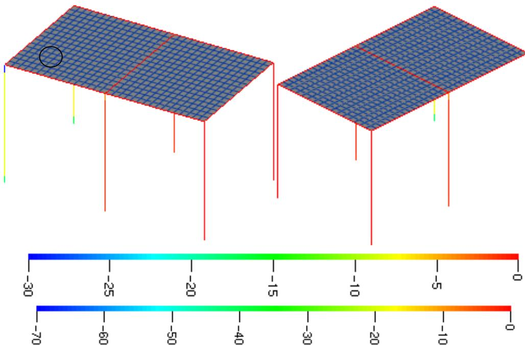
Fig. 19 The inertia moment change in the updated model for the second damage case
