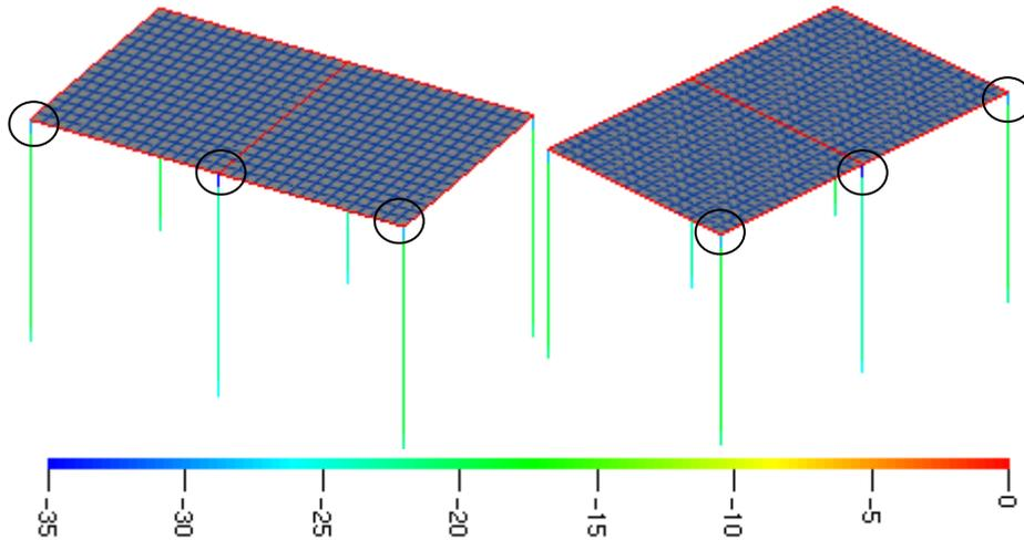
Fig. 18 The inertia moment change in the updated model for the first damage case
