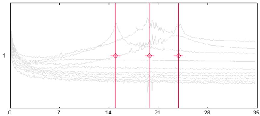
Fig. 8 The singular values diagram for the undamaged building model
