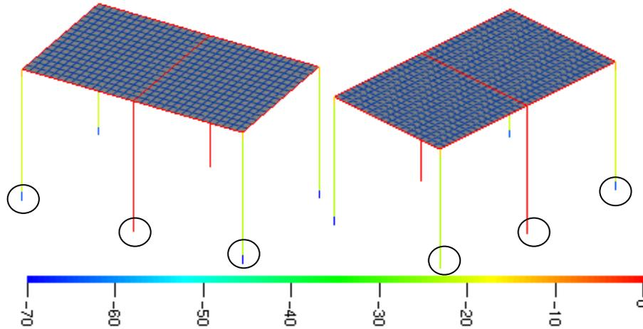
Fig. 19 The inertia moment change in the updated model for the second damage case
