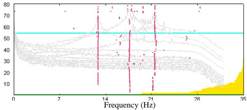
Fig. 12 The stabilization diagram for the first damage case of the building model
