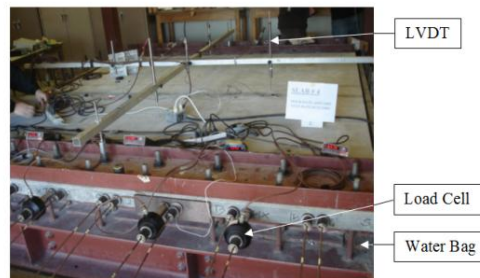
Fig. 3 Test set-up for one-way slabs (PTS-4) under uniformly distributed pressure (Bottom: fixed support end; top: pin support end)
