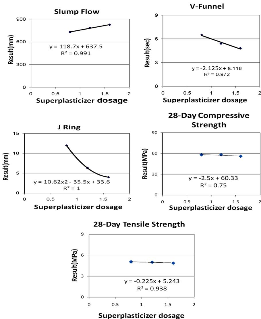
Fig. 1 Test results versus superplasticizer dosage of concrete mix one (W/C = 0.35, OPC)
