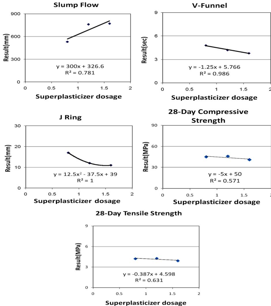
Fig. 4 Test results versus superplasticizer dosage of concrete mix four (W/C=0.45, SF10)
