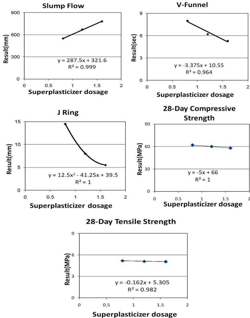
Fig. 2 Test results versus superplasticizer dosage of concrete mix two ( $W/C = 0.35$ , SF10)
