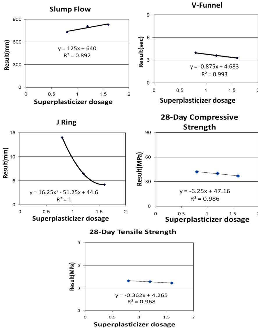
Fig. 3 Test results versus superplasticizer dosage of concrete mix three (W/C = 0.45, OPC)
