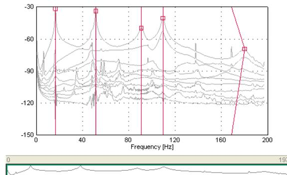
Fig. 5 SVSDM and AASD of the data set for plane frame
