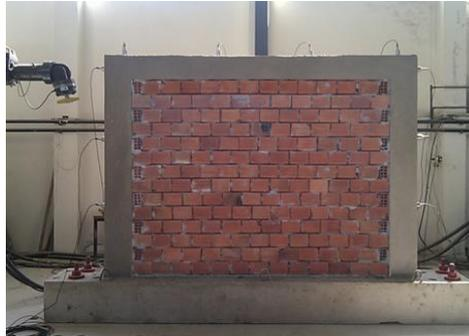
Fig. 7 A scene from ambient vibration tests of brick in-filled frame
