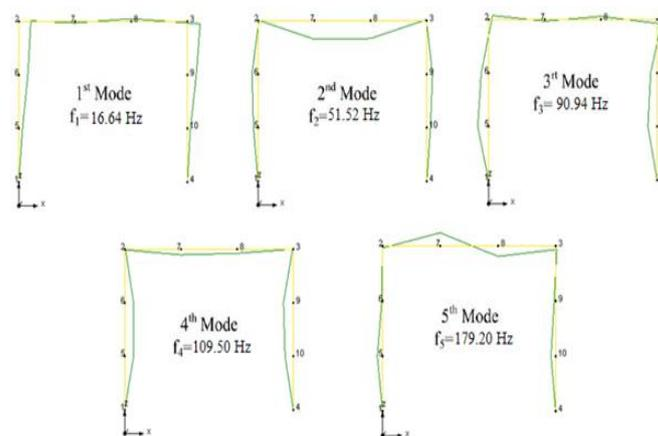
Fig. 6 The first five modes shapes of plane frame
