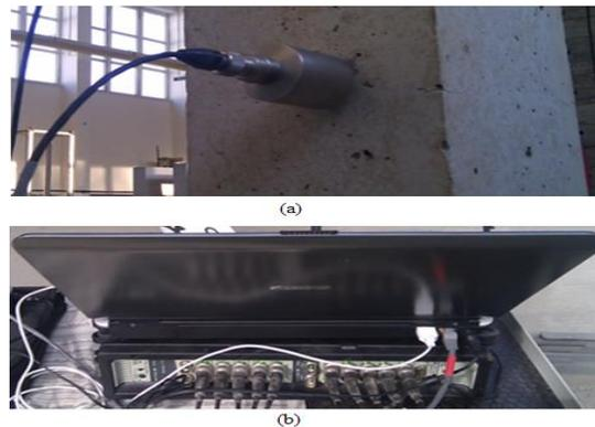
Fig. 2 Accelerometers and data acquisition system used for OMA
