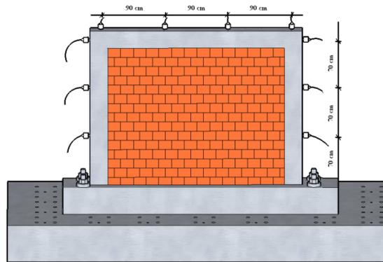
Fig. 8 Schematic views of accelerometer locations
