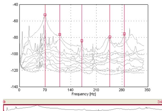
Fig. 13 SVSDM and AASD of the data set for brick in-filled with plaster frame
