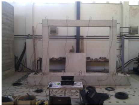
Fig. 3 A scene from ambient vibration tests of plane frame
