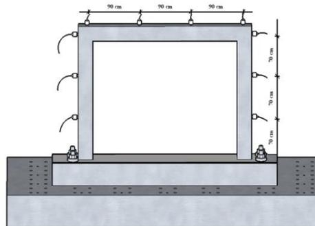
Fig. 4 Schematic views of accelerometer locations
