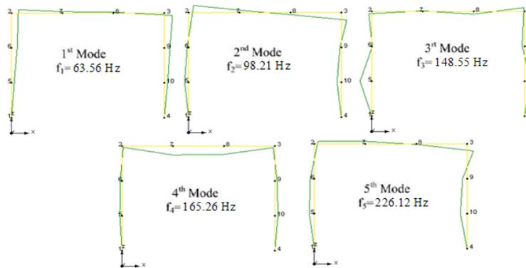
Fig. 10 The first five modes shapes of plane frame
