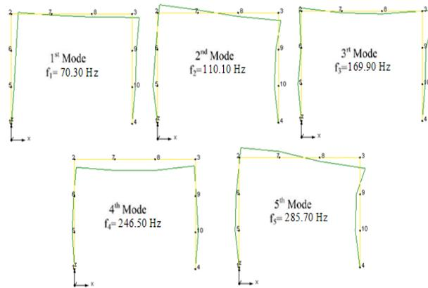
Fig. 14 The first five mode shapes of brick in-filled with plaster frame
