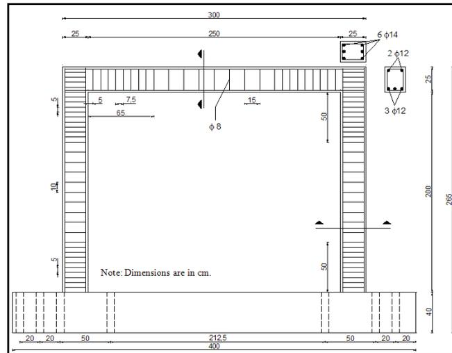
Fig. 1 Dimensions and reinforcement details of the RC frame
