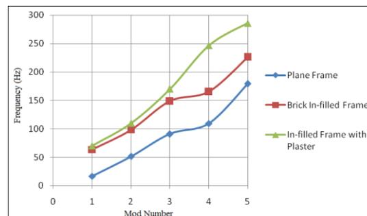
Fig. 15 Changing of the natural frequencies during construction stages
