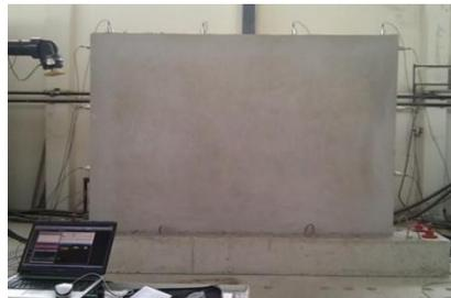
Fig. 11 A scene from ambient vibration tests of brick in-filled with plaster frame
