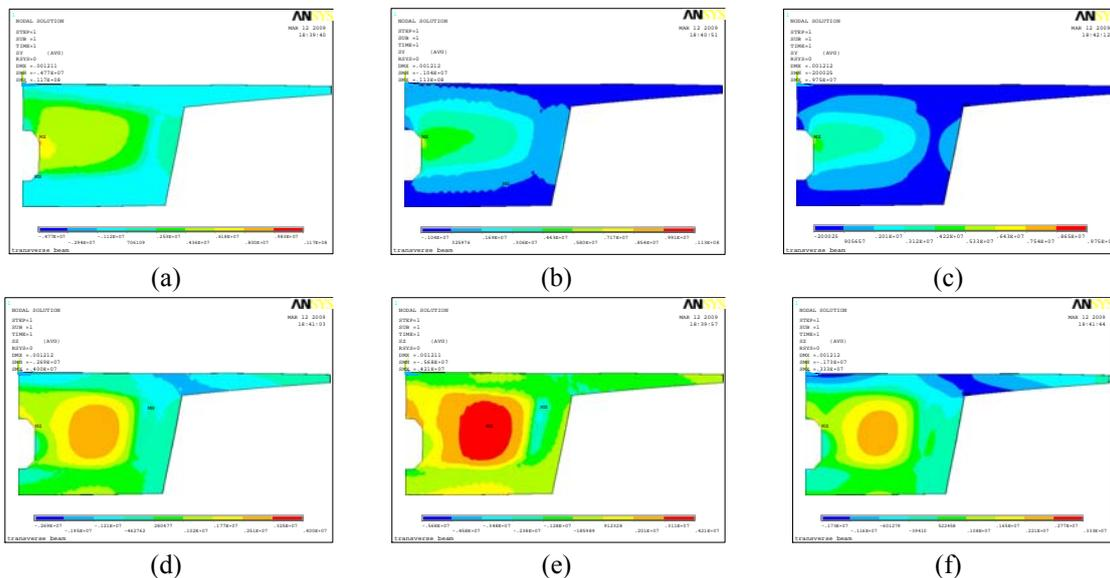
Fig. 9 Stress distribution under the first condition: (a) vertical stress in section 1#, (b) vertical stress in section 2#, (c) vertical stress in section 3#, (d) transverse stress in section 1#, (e) transverse stress in section 2# and (f) transverse stress in section 3#
