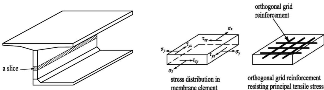
Fig. 2 Shear resistance distribution in membrane element
