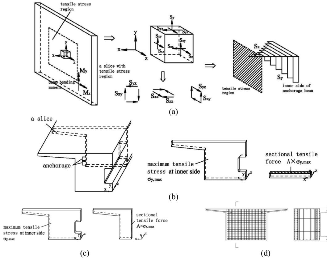
Fig. 3 Tensile stress method reinforcement: (a) tensile stress region of slices, (b) vertical tension force, (c) transverse tension force and (d) layout of reinforcements inside anchor cross beam
