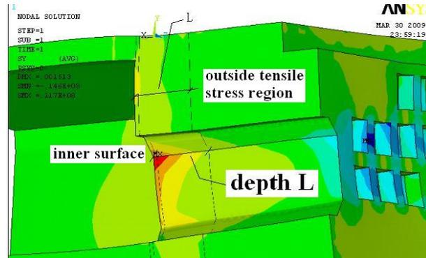
Fig. 4 Depth of tensile stress region
