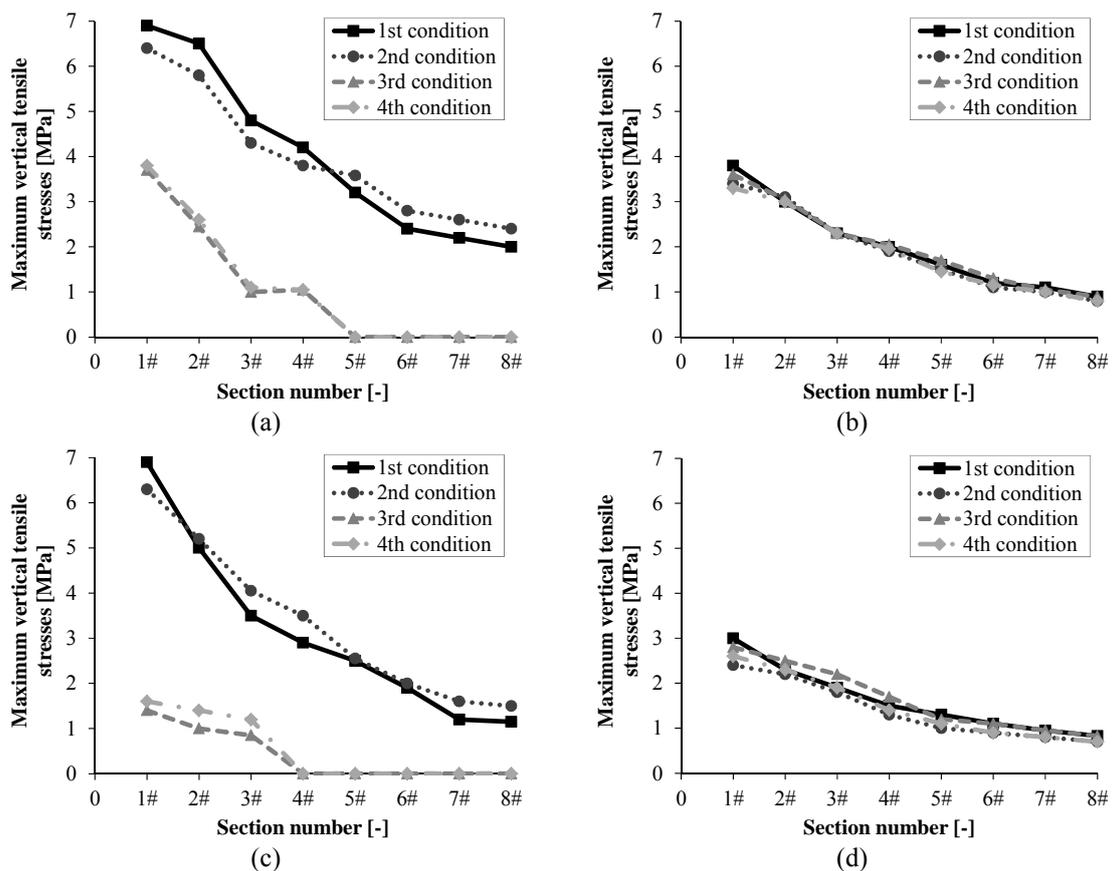
Fig. 11 Distributions of maximum tensile stresses in cross beam: (a) distributions of maximum vertical tensile stresses for anchorage assembly 1, (b) distributions of maximum transverse tensile stresses for anchorage assembly 1, (c) distributions of maximum vertical tensile stresses for anchorage assembly 2 and (d) distributions of maximum transverse tensile stresses for anchorage assembly 2
