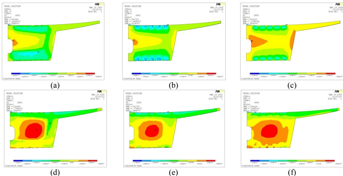
Fig. 10 Stress distribution under the fourth condition: (a) vertical stress in section 1#, (b) vertical stress in section 2#, (c) vertical stress in section 3#, (d) transverse stress in section 1#, (e) transverse stress in section 2# and (f) transverse stress in section 3#
