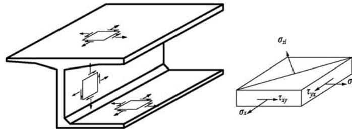
Fig. 1 Tensile stress region for elements under combined shear and bending loading
