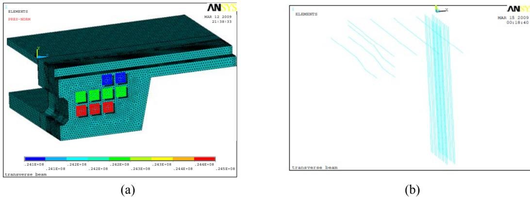
Fig. 8 Finite element model: (a) ANSYS model and (b) elements of transverse and vertical prestressing struts/tendons
