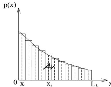
Fig. 5 Function of the depth of tensile stress region
