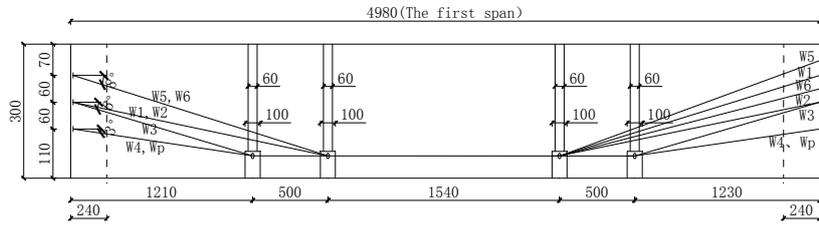
Fig. 6 Layout of external prestressing tendons
