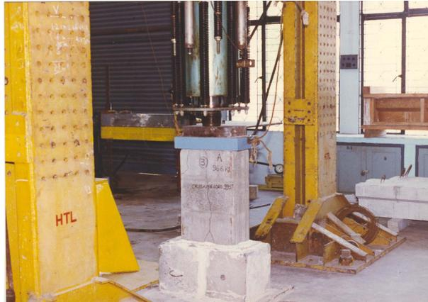
Fig. 2 Failure pattern of grouted HCB prism
