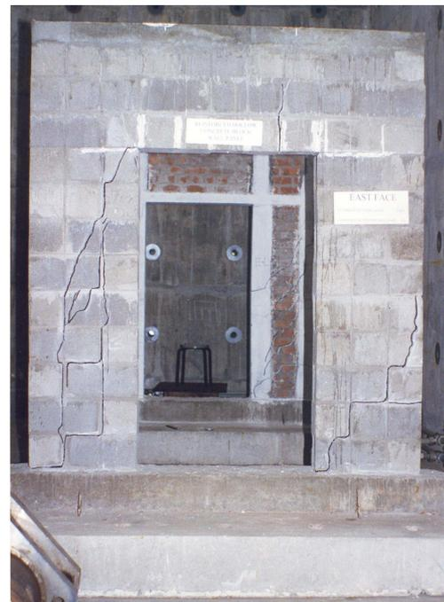
Fig. 7 Failure pattern of OP-HCB wall panel
