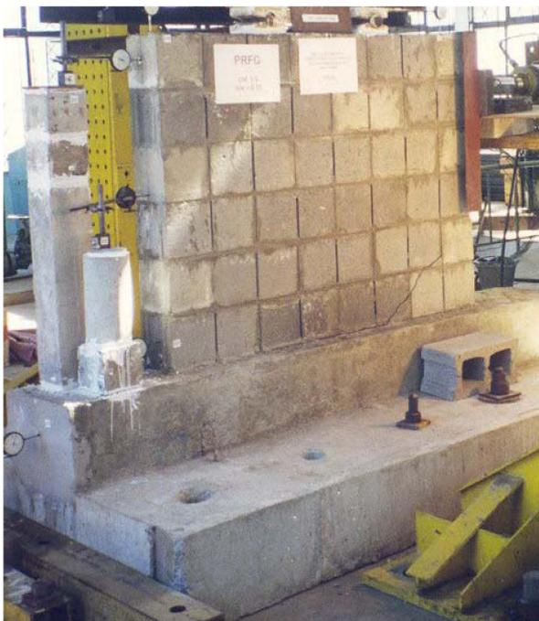
Fig. 6 Failure pattern of PR2-HCB wall panel
