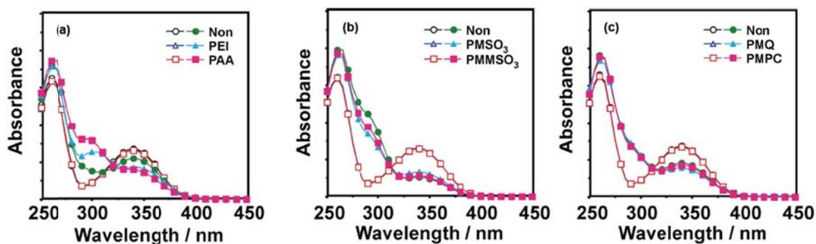
Fig. 5 Effect of the addition of various polymers on the NADH stability. The polymers used were (a) 0.1 wt% PEI and PAA; (b) 1 wt% PMSO<sub>3</sub> and PMMSO<sub>3</sub>; (c) 1 wt% PMQ and PMPC. The storage conditions were (a) pH 7.9 at 25°C for 7 days; (b) pH 7.5 at 25°C for 8 days; (c) pH 7.6 at 37°C for 7 days. The open and solid symbols represent the absorption spectra of NADH in various polymer solutions before and after incubation
