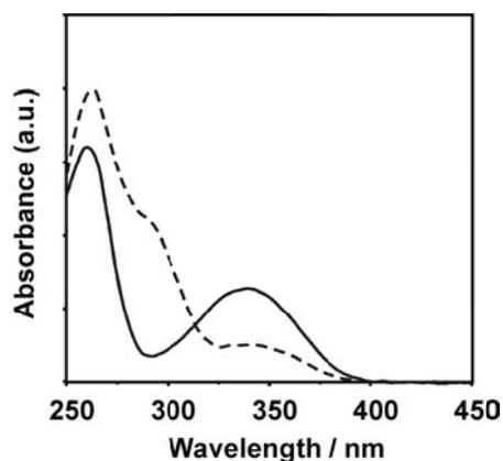
Fig. 3 UV spectra of NADH in 50 mM Tris buffered solution (pH 7.5). Before (solid line) and after a 7-day-incubation at 37°C (dotted line) are indicated
