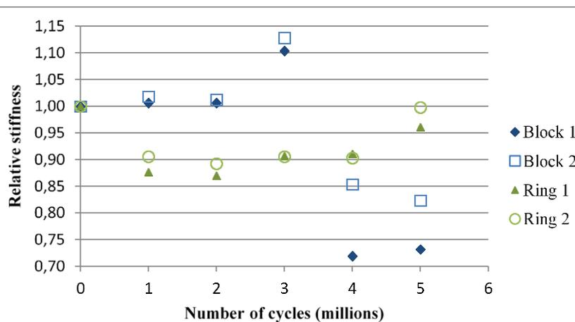
Fig. 7 Changes in stiffness of dampers and rings
