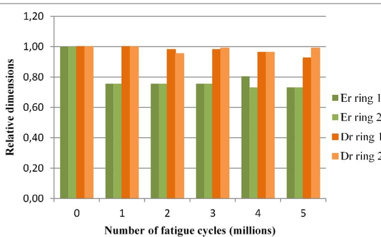
Fig. 6 Changes in relative dimensions of rings
