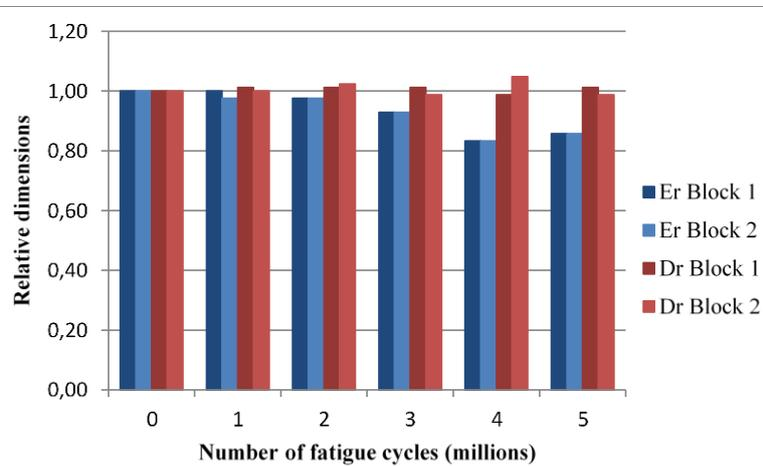
Fig. 5 Changes in dimensions of dampers
