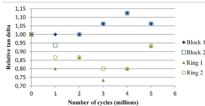
Fig. 8 Changes in  $\tan\delta$  of dampers and rings
