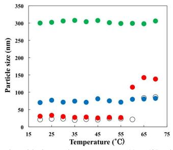
Fig. 3 Change in particle size over the temperature range 20 to 70°C. Poly(HEAA):  $\circ$ , PH<sub>99</sub>T<sub>11</sub>: •, PH<sub>92</sub>T<sub>9</sub>: •, PH<sub>99</sub>T<sub>52</sub>: •
