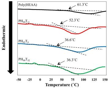
Fig. 2 DSC thermograms of lyophilized poly(HEAA) and PHT copolymers
