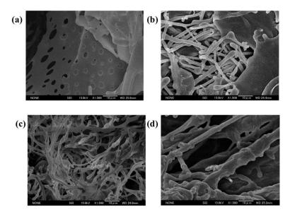
Fig. 1 SEM images of the freeze-dried polymers (Scale bar, 10  $\mu$ m): (a) Poly(HEAA), (b) PH<sub>99</sub>T<sub>11</sub>, (c) PH<sub>92</sub>T<sub>9</sub>, (d) PH<sub>99</sub>T<sub>52</sub>
