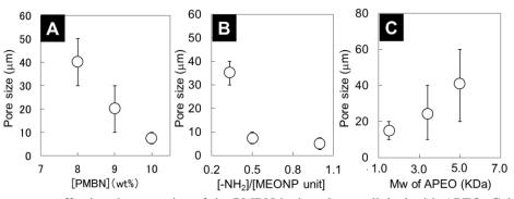
Fig. 8 Parameters affecting the pore size of the PMBN hydrogel cross-linked with APEO. Gelation was carried out at  $37^{\circ}$ C. Pore size of the PMBN hydrogels depended on [PNBN] (a), [-NH<sub>2</sub>/MEONP unit] (b), and Mw of APEO (c)
