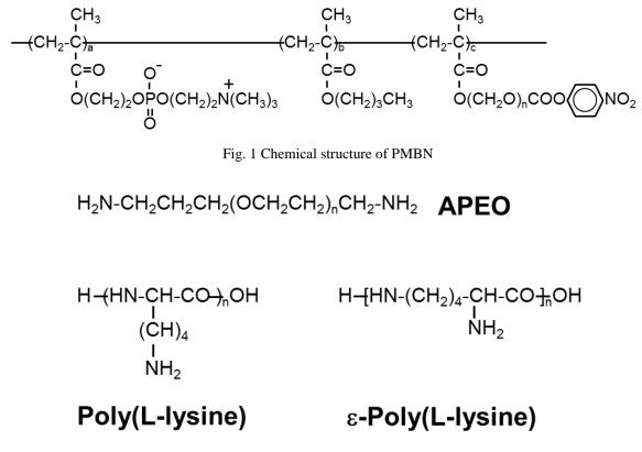
Fig. 2 Chemical structure of polymeric amine compounds as cross-linking agents
