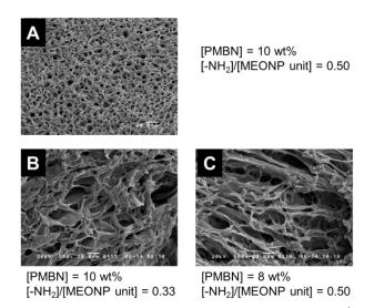
Fig. 6 SEM pictures of PMBN hydrogel cross-linked with APEO ( $Mw=1.5\times10^3$ ). Cross-linking reaction was carried out at 37 °C. a: [PMBN]=10 wt%, [-NH<sub>2</sub>]/[MEONP unit]=0.50; b: [PMBN]=10 wt%, [-NH<sub>2</sub>]/[MEONP unit]=0.33; c: [PMBN]=8 wt%, [-NH<sub>2</sub>]/[MEONP unit]=0.50
