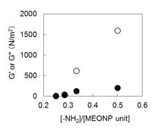
Fig. 5  $[-NH_2]/[MEONP unit]$  ratio dependence on G' and G'' of PMBN hydrogel cross-linked with APEO. Reaction was carried out at 37°C. Open circle: G' elastic modulus; closed circle: G'' loss modulus
