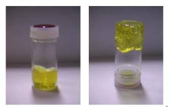
Fig. 3 PMBN hydrogel cross-linked with APEO ( $Mw=1.5\times10^3$ )
