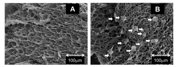
Fig. 9 SEM images of the PMBN hydrogel immobilized with glycine (a) and with the RGDS peptide (b) after culturing hydrogels with BPAEC for 48 h. The arrows represent adherent cells
