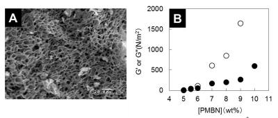
Fig. 7 (a) SEM pictures of PMBN hydrogel cross-linked with APEO ( $Mw=1.5\times10^3$ ) [PMBN]=8 wt% [-NH<sub>2</sub>]/[MEONP unit]=0.50, and (b) mechanical properties of the PMBN hydrogel with various concentrations of PMBN and [-NH<sub>2</sub>]/[MEONP unit]=0.50. The cross-linking reaction was carried out at 60°C. Open circle: G' elastic modulus; closed circle: G'' loss modulus
