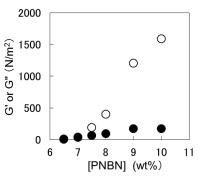
Fig. 4 PMBN concentration dependence on G' and G" of PMBN hydrogels cross-linked with APEO. The reaction was carried out at 37°C. Open circle: G' elastic modulus; closed circle: G" loss modulus
