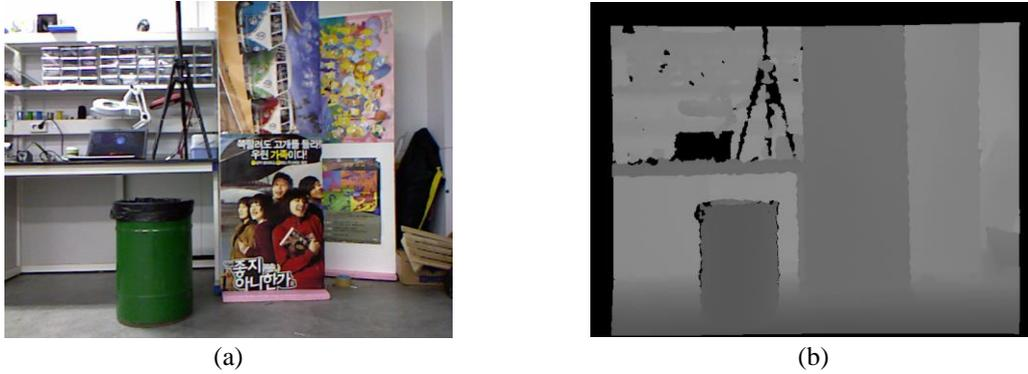
Fig. 1 RGB-D sensor data, (a) RGB color image and (b) Per-pixel depth data
