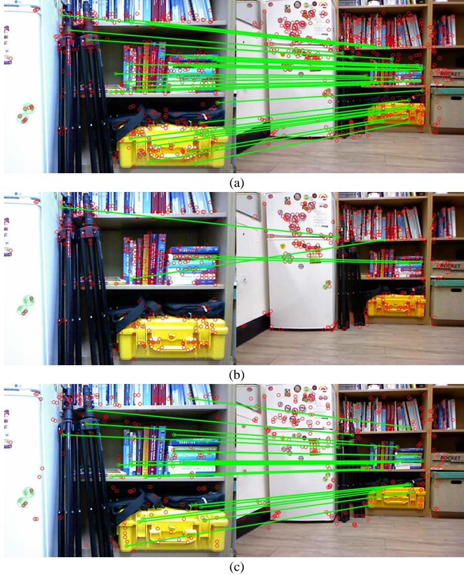
Fig. 9 Feature matching results, (a) Classical SURF (using four octaves), (b) Classical SURF (using one octave) and (c) DH-SURF
