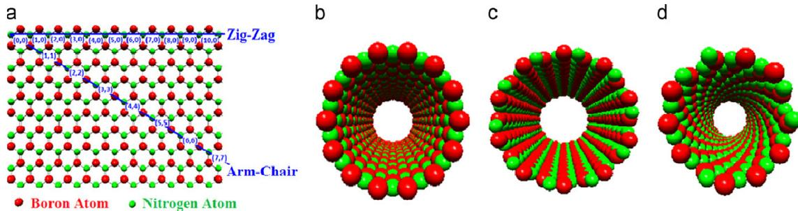
Fig. 1 (a) Plane BN sheet with possible wrapping of zigzag and armchair chiralities and structural models of single walled BNNTs made of a wrapped BN layer; (b) zigzag; (c) armchair; and (d) chiral (Panchal and Upadhyay 2013a)
