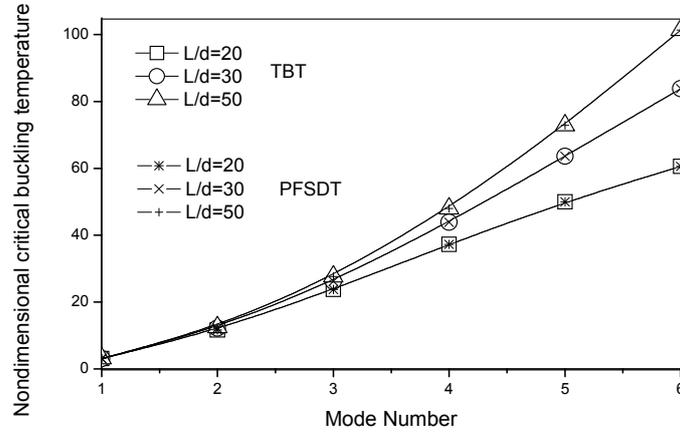
Fig. 3 Relation between the non-dimensional critical buckling temperature and the mode number for different values of  $L/d$  and  $e_0a = 0.4$  nm
