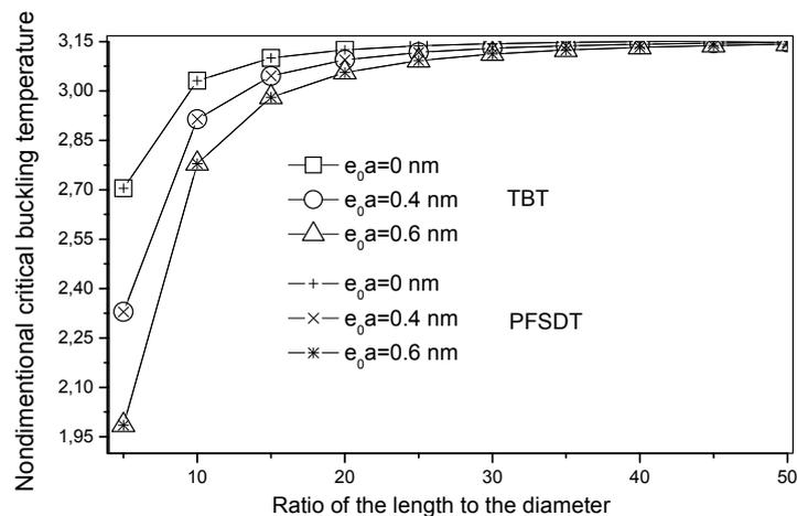
Fig. 4 Relation between the non-dimensional critical buckling temperature and  $L/d$  for different values of  $e_0a$  and  $n = 1$
