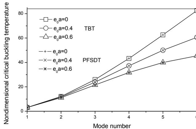
Fig. 2 Relation between the non-dimensional critical buckling temperature and the mode number for different scale coefficients ( $e_0 a$ ) and  $L/d = 20$
