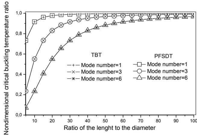
Fig. 5 Ratio of the critical buckling temperature by (TBT, PFSDT) to the nonlocal EBT vs. ratio of the length to the diameter for different mode numbers ( $e_0a = 0.6$  nm)
