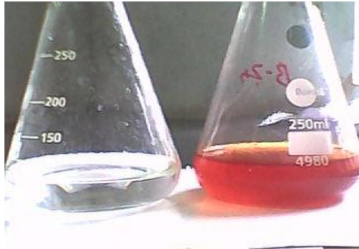
Fig. 1 Shows that \text{AgNO}_3 color changes from colorless to dark brown color (Synthesis of silver nanoparticles by Sodium citrate)
