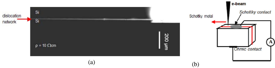
Fig. 3 Formation of a conducting channel along the dislocation network in the interface of a bonded Si wafer pair (a). EBIC micrograph. Sketch of the experimental setup (b)
