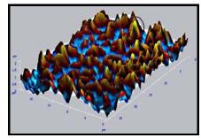
Fig. 1 AFM image of the microstructure of ZnO (in the circle the characteristic pyramidal shape). The pyramides tops exhibit negative and positive potential at opposite sides under deflection
