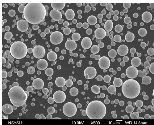
Fig. 3 SEM images of the  $\text{Fe}_{50}\text{Cr}_{24}\text{Mo}_{21}\text{Si}_2\text{B}_3$  powder particles
