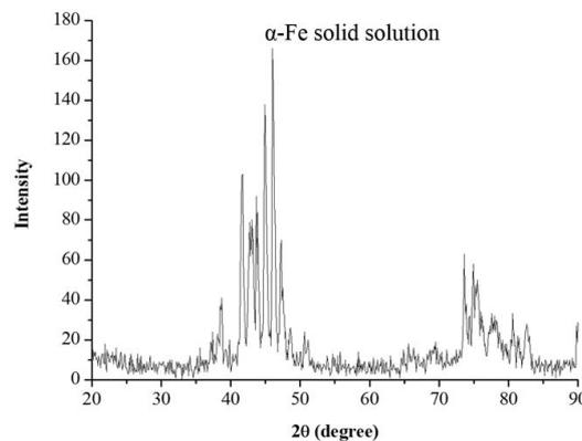
Fig. 2 X-ray diffraction pattern of the gas atomized powder particles
