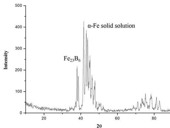
Fig. 1 X-ray diffraction pattern of the  $\text{Fe}_{50}\text{Cr}_{24}\text{Mo}_{21}\text{Si}_2\text{B}_3$  master ingot
