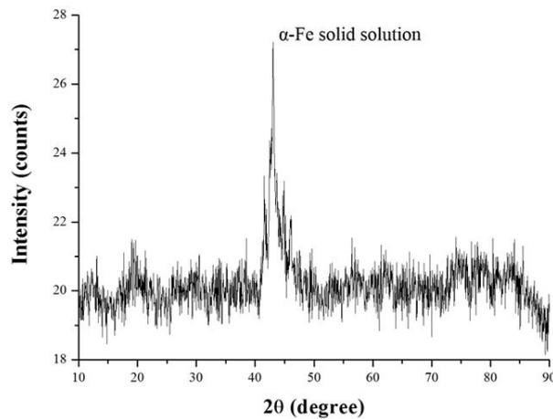
Fig. 4 X-ray diffraction pattern of Fe-based alloy coating
