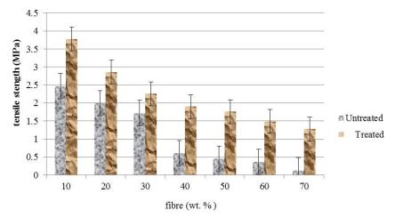
Fig. 1 Tensile strength of oil palm EFB reinforced polyest reinforced composites at different fibre loading
