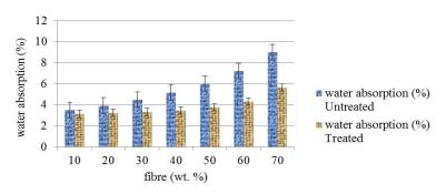
Fig. 4 Water absorption of oil palm EFB reinforced polyester reinforced composites at different fibre loading
