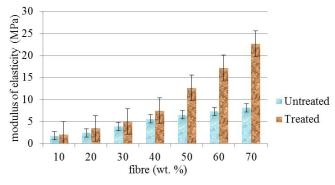
Fig. 2 Modulus of elasticity of oil palm EFB reinforced polyester reinforced composites at different fibre loading
