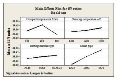
Fig. 1 Mean of S/N ratios for density of samples versus levels of input parameters
