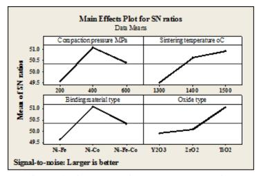
Fig. 3 Mean of S/N ratios for hardness of samples versus levels of input parameters
