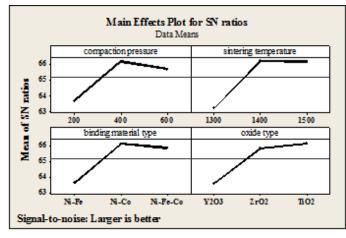
Fig. 4 Mean of S/N ratios for compressive strength of samples versus levels of input parameters
