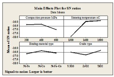
Fig. 2 Mean of S/N ratios for electrical conductivity of samples versus levels of input parameters
