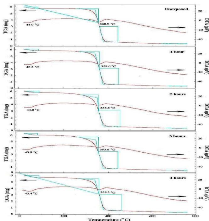
Fig. 4 TGA and DTA curves for unexposed and exposed HPMC films
