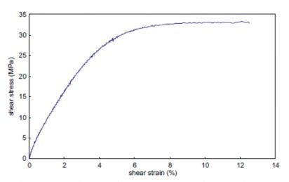
Fig. 2 Stress-strain curve of FM73M Epoxy adhesive (Oudad 2009)
