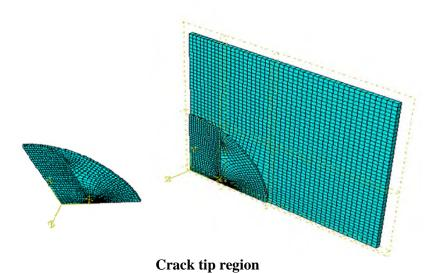
Fig. 3 Typical mesh model of the global structure and near the crack tip
