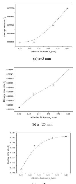
(c) a= 45 mm Fig. 5 Damage zone ratio vs adhesive thickness  $e_a$  (mm)
