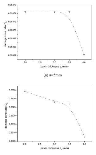
(b) a=25 mm Fig. 6 Damage zone ratio vs patch thickness e<sub>r</sub> (mm)
