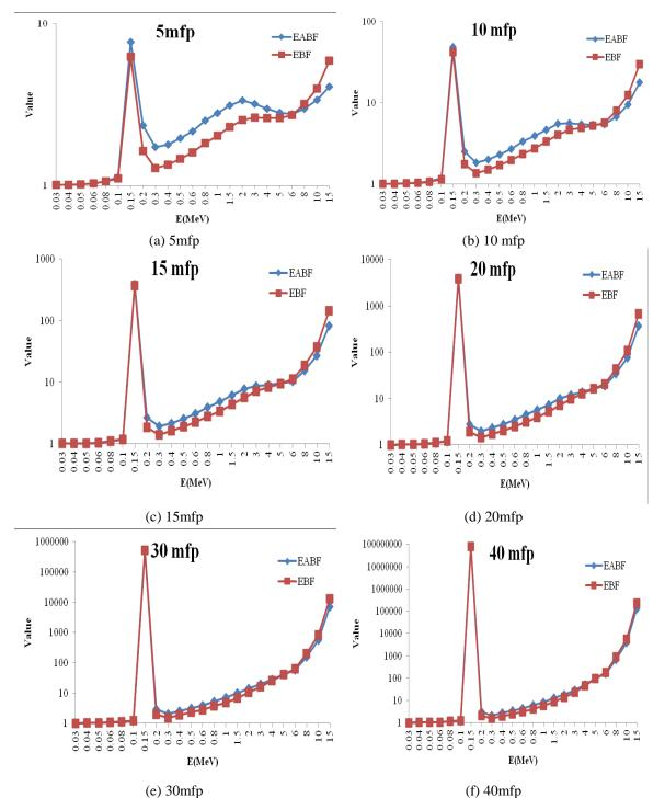
Fig. 1 Variation of EABF and EBF with incident photon energy (MeV) for uranium
