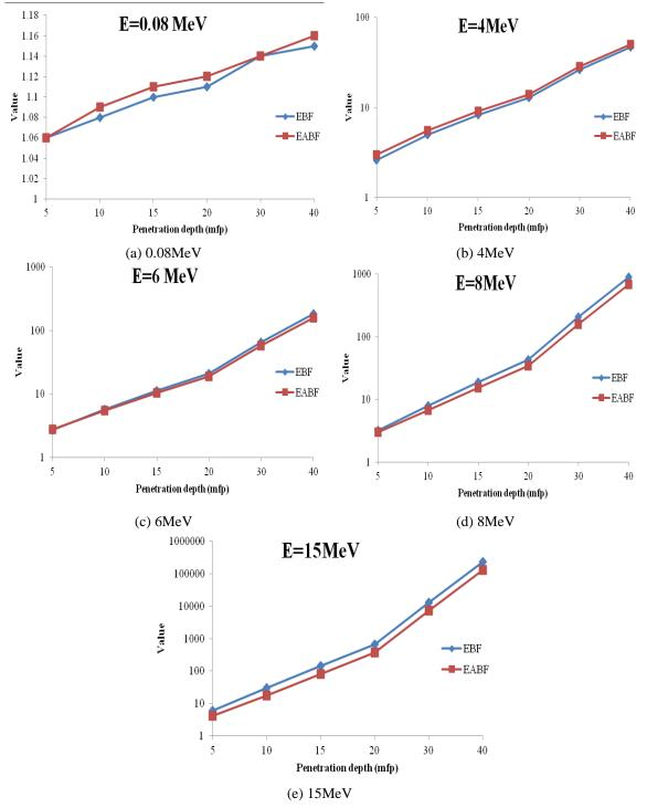
Fig. 2 Variation of EABF and EBF with penetration depth of uranium at energy ranges 0.08-15 MeV
