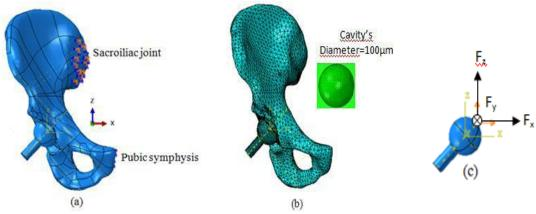
(a)Boundary condition and directions of forces applied to the center of femoral head
