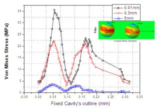
Fig. 9. Variation of the stress in cement around the mobile cavity according to the distance separating it to that fixed at the free edge both to the interface cement/bone
