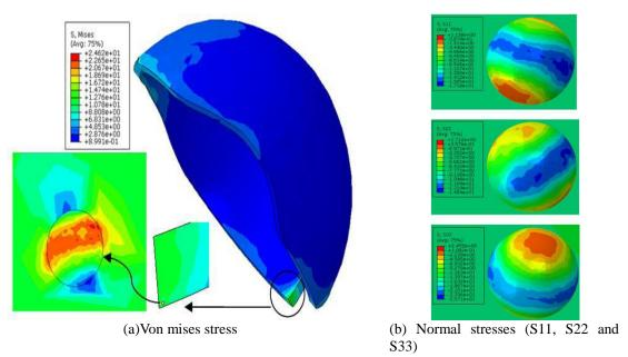
Fig. 5 Stress level and distribution in the cement around the cavity
