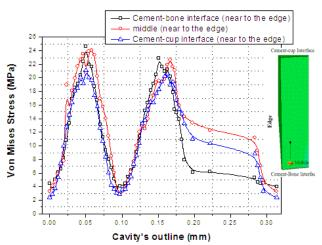
Fig. 7 Variation of the stress in the cement around the cavity according to its position along the thickness of the cement close to the edge
