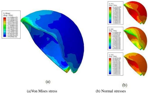
Fig.4 Stress level and distribution in the cement
