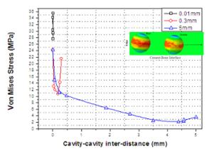
Fig. 10 Variation of the stress according to the fixed cavity- mobile cavity interdistance
