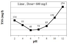
Fig. 3 The effect of changing pH on removal of TSS using 600 mg/1 lime
