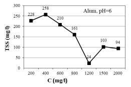
Fig. 2 The effect of changing alum concentration on TSS removal at pH=6
