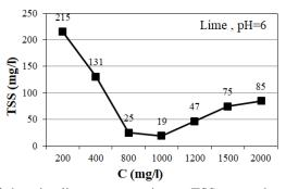
Fig. 4 The effects of changing lime concentration on TSS removal at pH=6 at TSS removal
