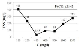
Fig. 6 The effects of changing FeCl<sub>3</sub> concentration on TSS removal at pH=2
