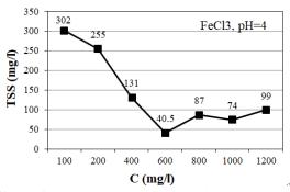
Fig. 7 The effects of changing FeCl<sub>3</sub> concentration on TSS removal at pH=4
