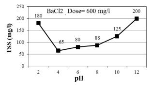
Fig. 10 The effect of changing pH 4 on TSS removal using 600 mg/l BaCl2
