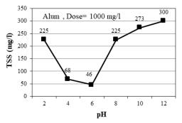
Fig. 1 The effect of changing pH on TSS removal using 1000 mg/1 Alum
