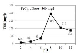
Fig. 5 The effects of changing pH on removal of TSS using 300 mg/l FeCl<sub>3</sub>
