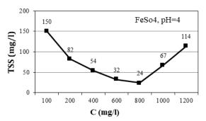
Fig. 9 The effect of changing FeSO4concentration on the TSS removal at pH=4
