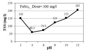
Fig. 8 The effect of changing pH on TSS removal using 300 mg/l FeSO4
