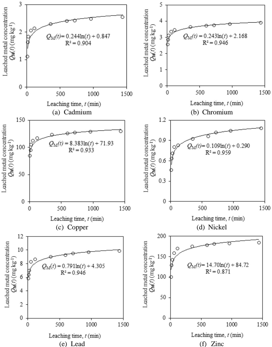
Fig. 1(a) Cumulative amounts (mg/kg) of heavy metals leached from water treatment sludge (solid/liquid ratio=1 g/50 mL) with time using 0.05 M EDTA along with curves from Elovich model
