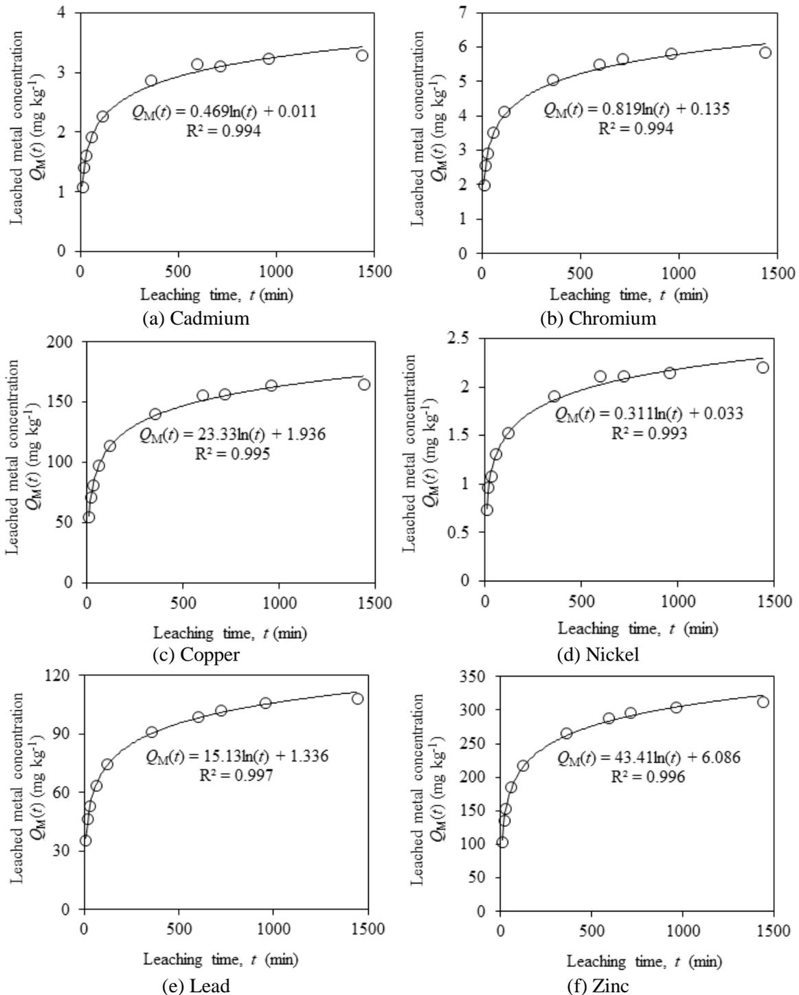
Fig. 1(b) Cumulative amounts (mg/kg) of heavy metals leached from wastewater treatment sludge (solid/liquid ratio=1 g/50 mL) with time using 0.05 M EDTA along with curves from Elovich model
