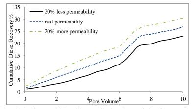
Fig. 7 Analysis of permeability effects on the diesel remediation from sand column (10000 ppm initial diesel concentration, 0.3 percent-mass SDS concentration)
