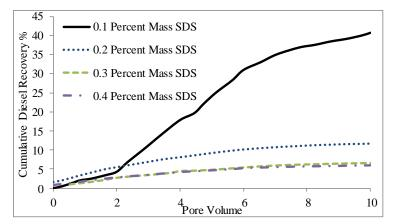
Fig. 4 Simulation results for diesel remediation with 20000 ppm concentration in soil column with different percent-mass of SDS
