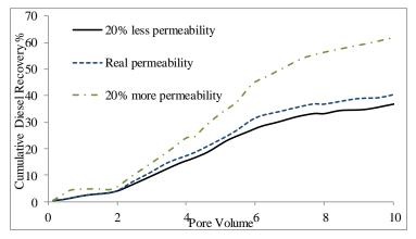
Fig. 8 Analysis of permeability effects on the diesel remediation from sand column (20000 ppm initial diesel concentration, 0.1 percent-mass SDS concentration)
