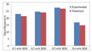
Fig. 5 Comparison between model prediction and experimental measurement for diesel removal (10000 ppm initial diesel concentration)
