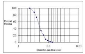
Fig. 2 Grain size distribution of sand which was used in the soil washing experiment
