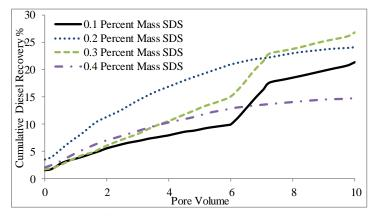
Fig. 3 Simulation results for diesel remediation with 10000 ppm concentration in soil column with different percent-mass of SDS
