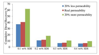
Fig. 10 Comparison between diesel removal efficiency of model by different permeability (with 20000 ppm initial diesel concentration)
