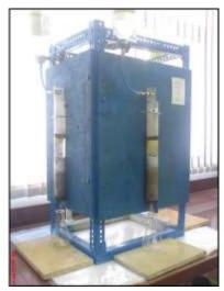
Fig. 1 Sand column apparatus of soil washing process (Salehian 2007)
