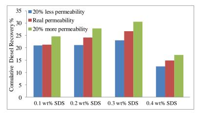
Fig. 9 Comparison between diesel removal efficiency of model by different permeability (with 10000 ppm initial diesel concentration)
