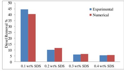
Fig. 6 Comparison between model prediction and experimental measurement for diesel removal (20000 ppm initial diesel concentration)
