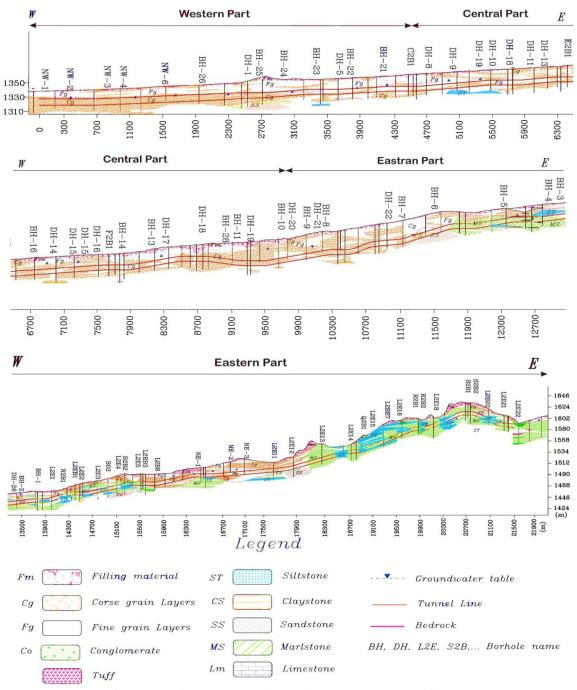
Fig. 9 Geological cross traced by boring results (Mohammadi 2015)
