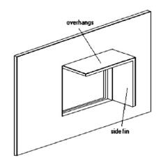
Fig. 2 Shading device configuration
