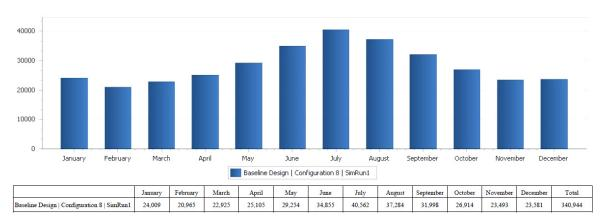
Fig. 9 Total monthly electrical consumption (kWh), After retrofit
