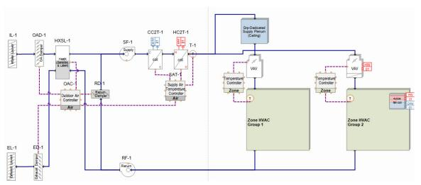
Fig. 5 Air loop block diagram
