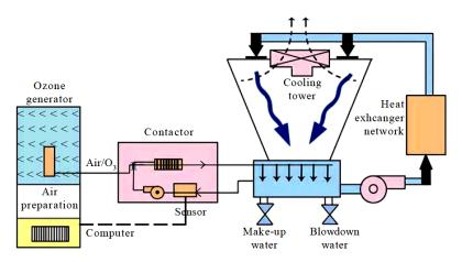
Fig. 1 A schematic of integrating ozone treatment into the cooling tower
