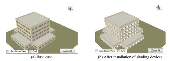
Fig. 3 Shading device configuration
