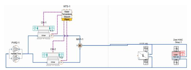
Fig. 6 Chilled water loop
