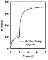
(a) Comparison between the experimental trend and the theoretical curves calculated from the Langmuir, BDDT and two-step Langmuir equations with the parameters given in Table A5
