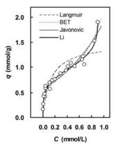
Fig. 4 Type II isotherm of the sorption of phenol on activated carbon showing comparison between the experimental trend and the theoretical curves calculated from the Langmuir, BET, Jovanović and Li equations with the parameters given in Table A3 (Data of Miller and Clump (1970))
