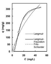
Fig. 7 Type V isotherm of the sorption of fluoride on MgAl-CO<sub>3</sub> layered double hydroxides showing comparison between the experimental trend and the theoretical curves calculated from the Langmuir, Langmuir-Freundlich and Fritz-Schlunder equations with the parameters given in Table A7 (Data of Lv *et al.* (2007))
