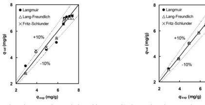
(a) Comparison between the methylene blue data of Fig. 2 and *q* values calculated from the Langmuir, Langmuir-Freundlich and Fritz-Schlunder equations with the parameters given in Table A1
