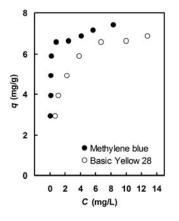
Fig. 2 Type I isotherms of the sorption of methylene blue and basic yellow 28 on natural phosphate rock (Data of Barka *et al.* (2009))
