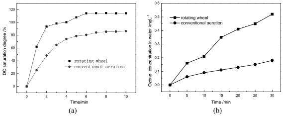
Fig. 2 Comparison of two gas transfer methods for manufacturing high stability of (a) dissolved oxygen; and (b) ozone in water
