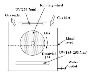
Fig. 1 Schematic diagram of rotating wheel reactor for manufacturing high concentration and high stability of dissolved gases in water
