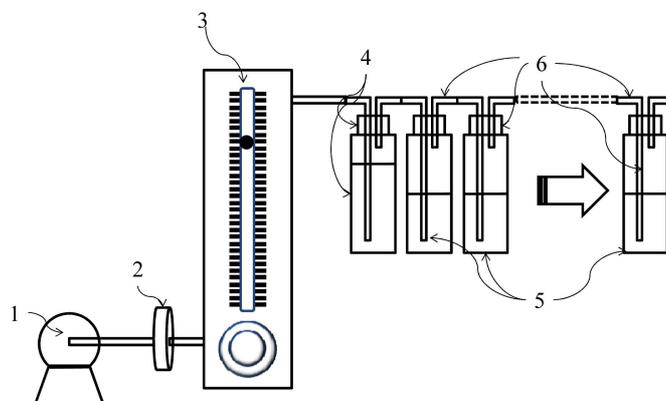
Fig. 1 Experimental apparatus for air sparging system (① Air blower; ② 0.2  $\mu\text{m}$  Filter; ③ Flow meter; ④ Humidifier; ⑤ Soil slurry vials; ⑥ Air flow tubes)
