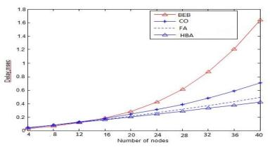
Fig. 5 Nodes vs Transmission delay at different broadcast algorithm
