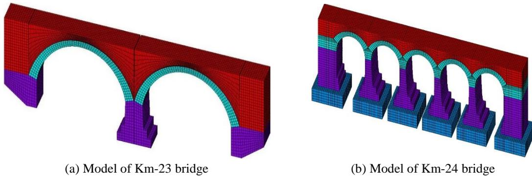
Fig. 2 3D Finite element model and boundary conditions
