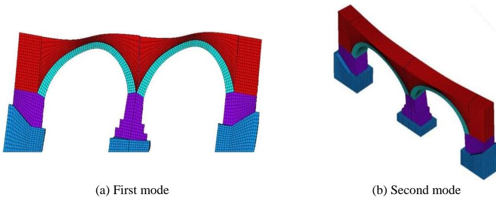
Fig. 3 Displacement correlated to km-23 bridge
