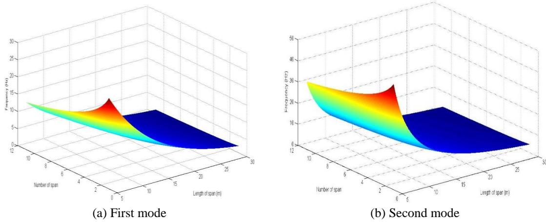
Fig. 8 The effects of span length and the number of span on frequencies of the plain concrete arch bridges. (a) the first mode, and (b) the second mode
