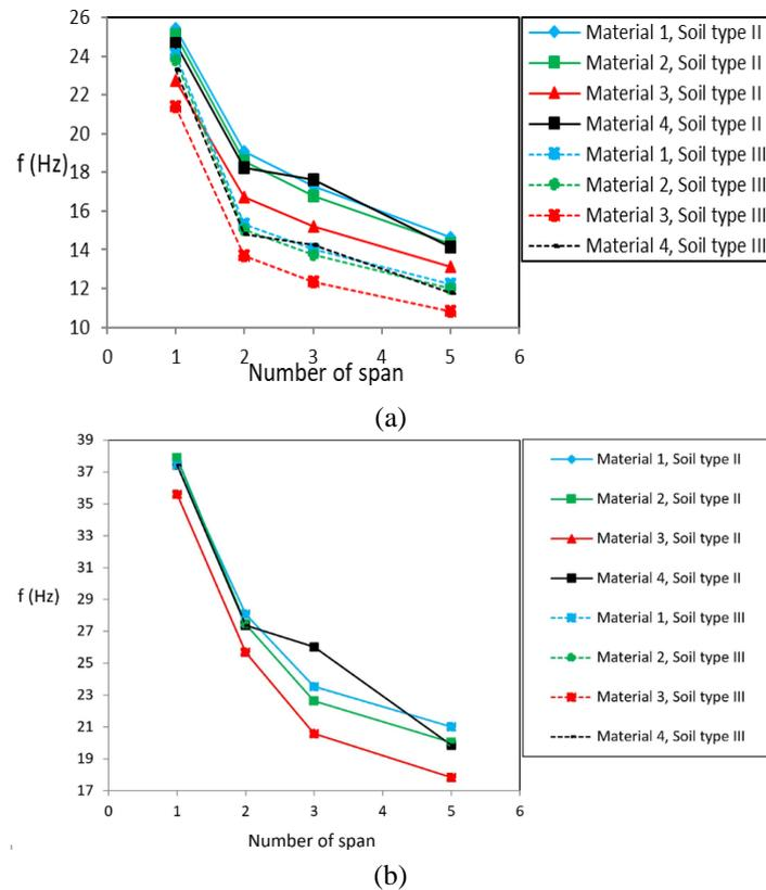
Fig. 6 Computed frequencies of the Km-24 bridge. (a) first mode, and (b) second mode
