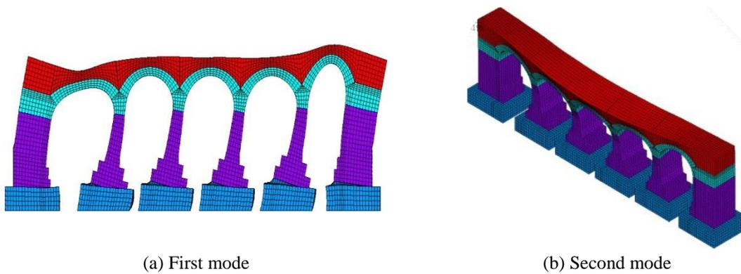
Fig. 4 Displacement correlated to km-24 bridge
