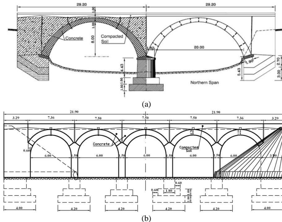
Fig. 1 Geometric characteristics of bridges (Marefat *et al.* 2004): (a) km-23 bridge and (b) km-24 bridge (units are in meter)
