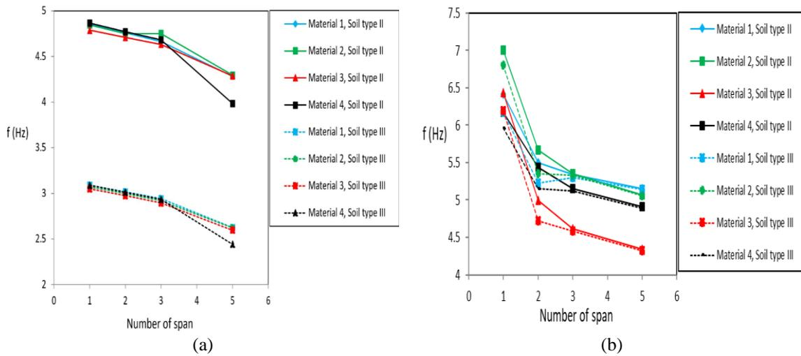
Fig. 5 Computed frequencies of the Km-23 bridge. (a) first mode, and (b) second mode
