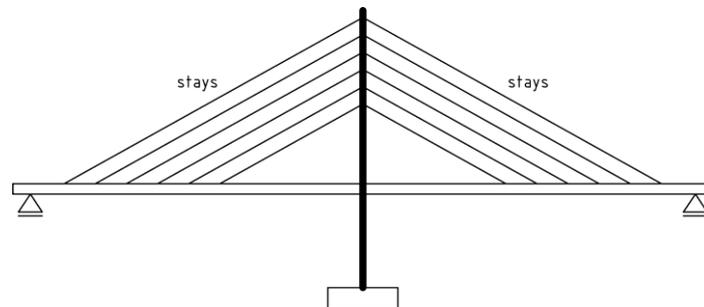
Fig. 5 A diagram of a typical cable-stayed footbridge
