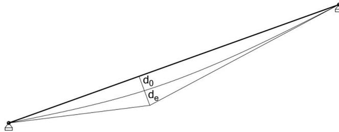
Fig. 12 Additivity of the stay cable deflections for the loads exerted by the weight of the bridge itself and the force  $F$
