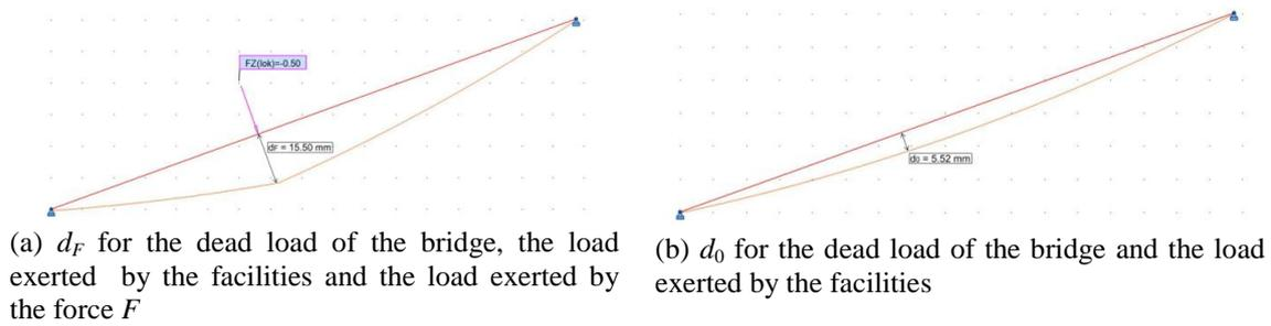
Fig. 14 Deformations of cable 2W determined numerically
