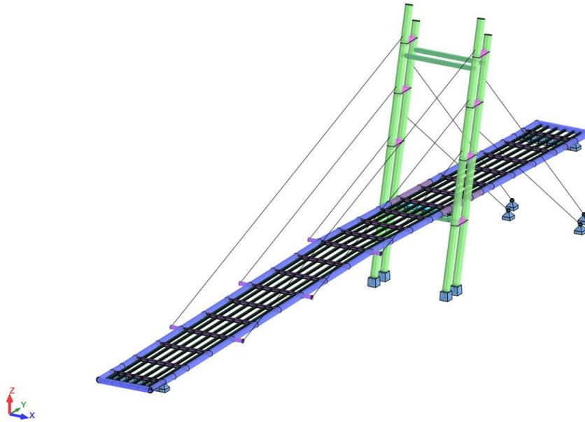
Fig. 15 A numerical model of the footbridge
