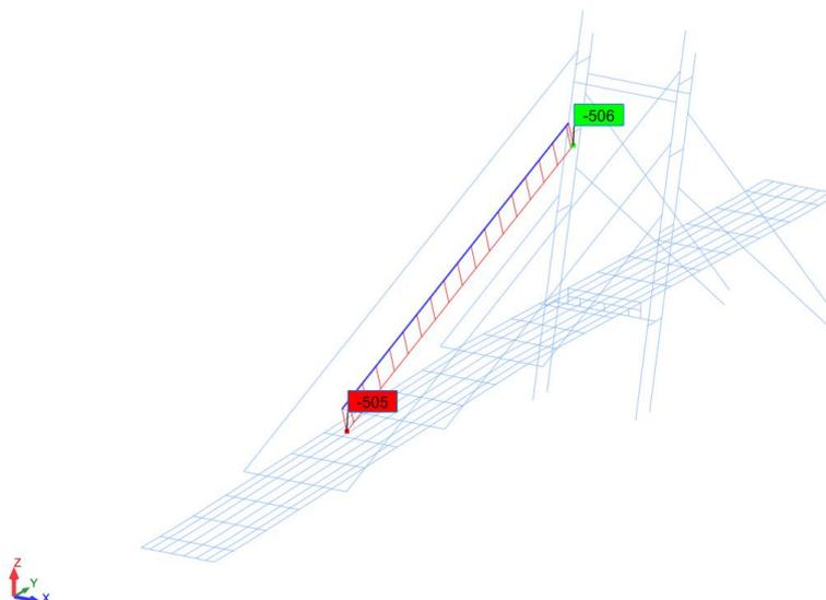
Fig. 16 Stresses in cable 2W determined through 3D analysis ( $\sigma = \sigma_s = 506$  MPa)
