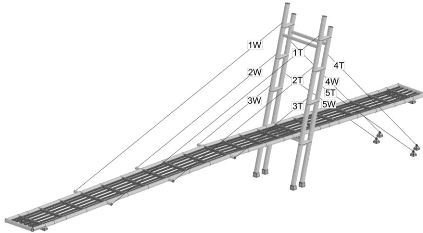
Fig. 11 Cables anchored to the deck (numbered 1W-5W) and cables anchored to the ground (numbered 1T-5T)
