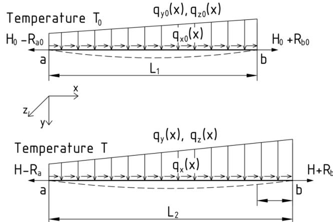
Fig. 3 The behaviour of a stay
