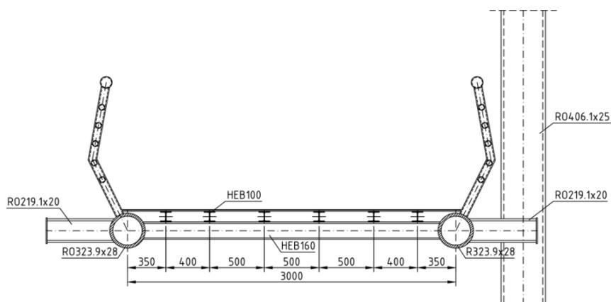
Fig. 10 A cross-sectional view of the load-carrying system of the footbridge (based on Biliszczyk *et al.* 2001)
