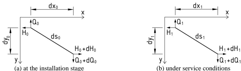
Fig. 2 The behaviour of an elementary section of a high tension cable
