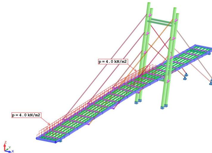
Fig. 17 An example of live load acting on the footbridge
