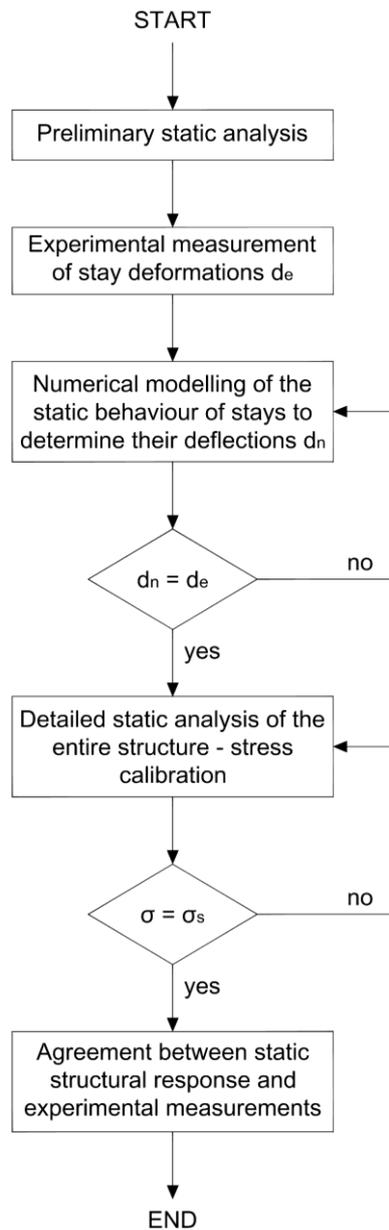
Fig. 4 The algorithm of the experimental and numerical method for assessing the structural response of cable-stayed footbridges
