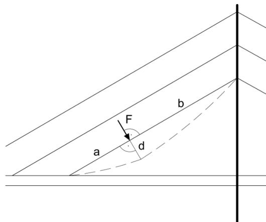
Fig. 6 Load  $F$  applied to a stay and the principle of measurement of the deflection  $d$
