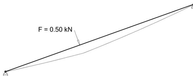
Fig. 13 The statics of stay 2W deformed under the load  $F$
