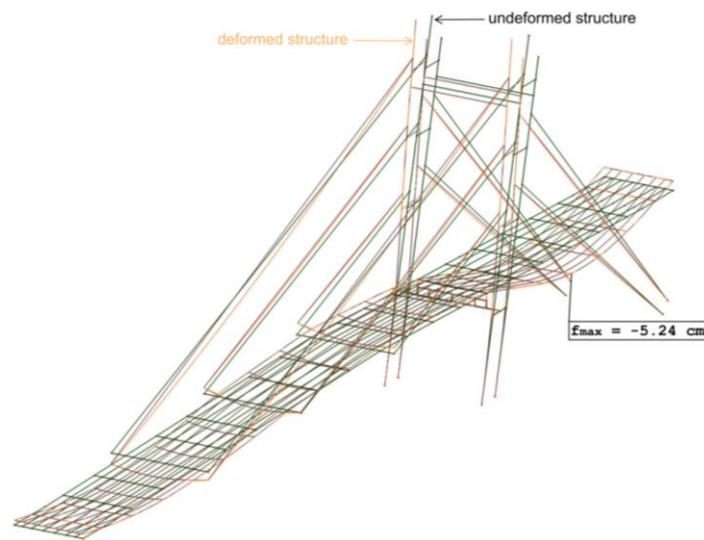
Fig. 18 A representation of the extreme deformations of the footbridge
