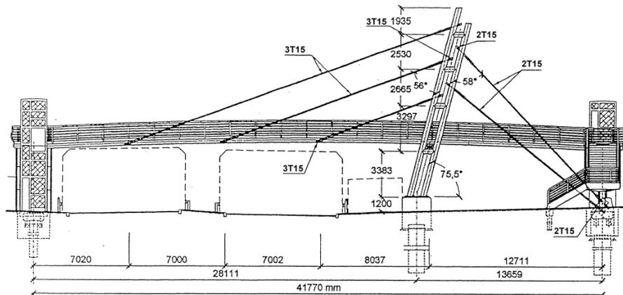
Fig. 9 A side view of the footbridge structure (Biliszczuk *et al.* 2001)
