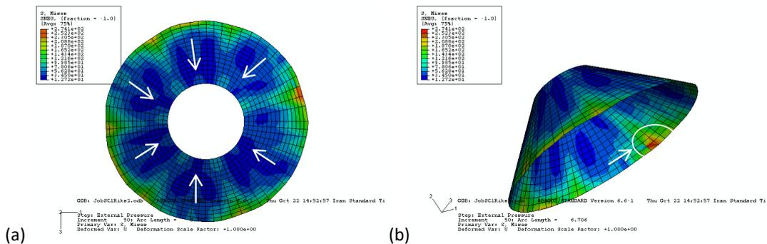
Fig. 5 Stress distribution and creation of the buckling lodes in the SCS model with no dent
