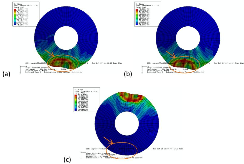
Fig. 6 Stress distribution in the zone of dent imperfection for the model SCS: Figures a to c represent inclined, horizontal and vertical dents respectively
