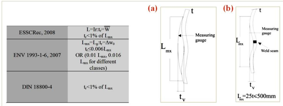
Fig. 4 Tolerated imperfections based on available design codes. (a) Dimple in vertical direction, (b) dimple of hoop direction (Maali *et al.* 2012).
