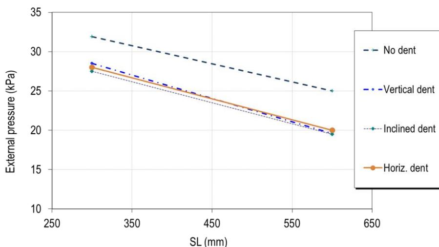
Fig. 2 Critical load of the truncated cones, intact and dented shells
