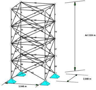
Fig. 3 Seventy-two bar truss
