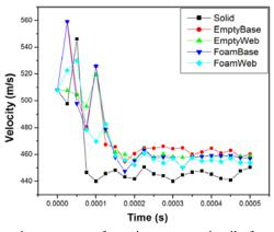
Fig. 11 Velocity-time response for ogive-nose projectile for a varied impact
