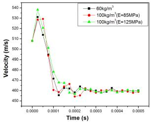
Fig. 9 Velocity-time response for projectile impacting on PVC foam core corrugated sandwich plate
