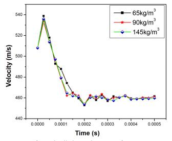
Fig. 8 Velocity-time response for projectile impacting on PU foam core corrugated sandwich plate
