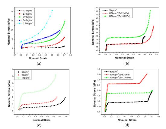
Fig. 2 Stress-strain curve of different foams; (a) Aluminum, (b) PMI, (c) PU and (d) PVC under uniaxial compression loading
