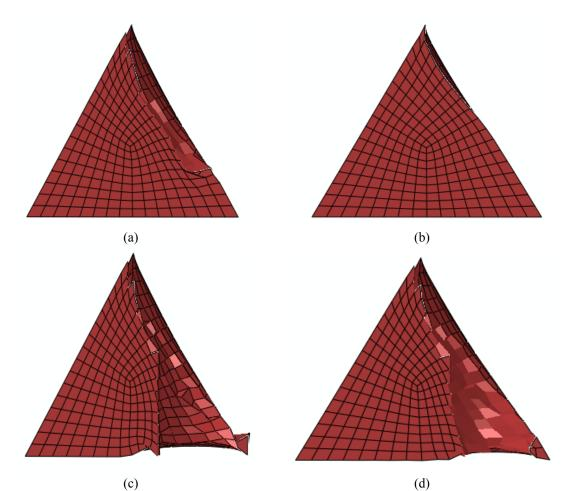
Fig. 5 Foam failure on web impact at different time interval; (a) 25µs, (b) 75µs, (c) 150 µs and (d) 200µs
