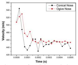
Fig. 13 Comparison of velocity-time response for conical-nose and ogive-nose projectile due to web impact
