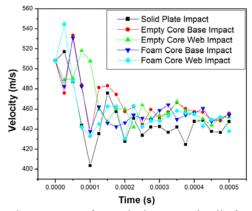
Fig. 12 Velocity-time response for conical-nose projectile for a varied impact
