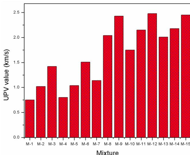
Fig. 4 Effect of coal bottom ash on UPV of coal ash bricks
