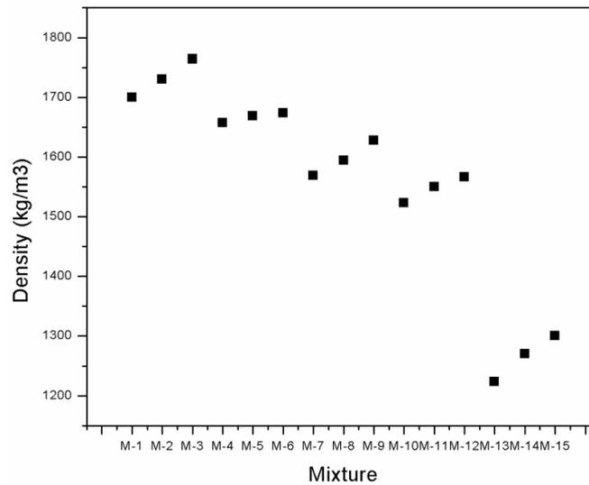
Fig. 1 Effect of coal bottom ash on density of coal ash bricks
