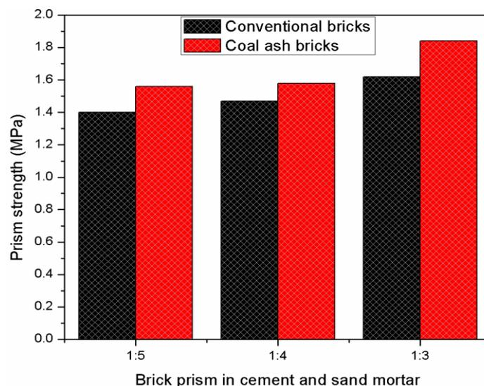
Fig. 6 Effect of coal bottom ash on masonry prism strength of coal ash bricks
