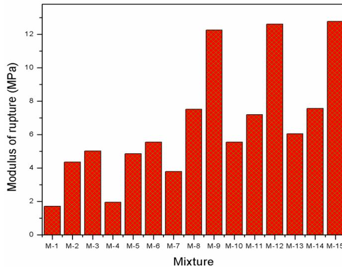
Fig. 3 Effect of coal bottom ash on modulus of rupture of coal ash bricks
