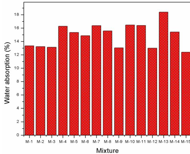
Fig. 5 Effect of coal bottom ash on water absorption of coal ash bricks
