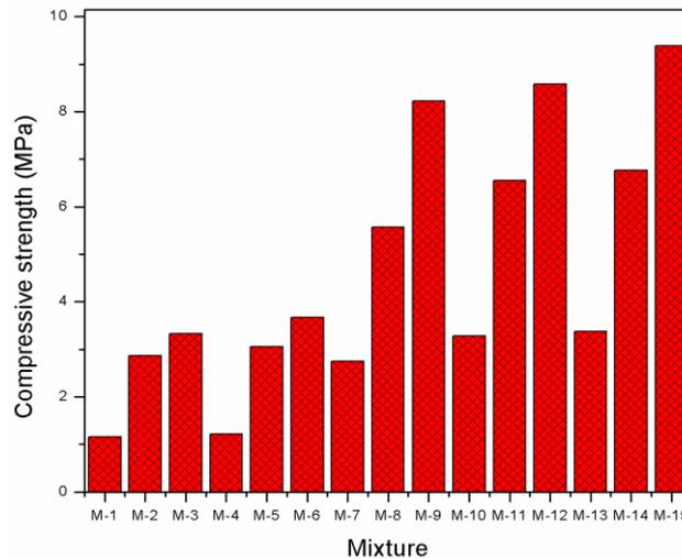
Fig. 2 Effect of coal bottom ash on compressive strength of coal ash bricks
