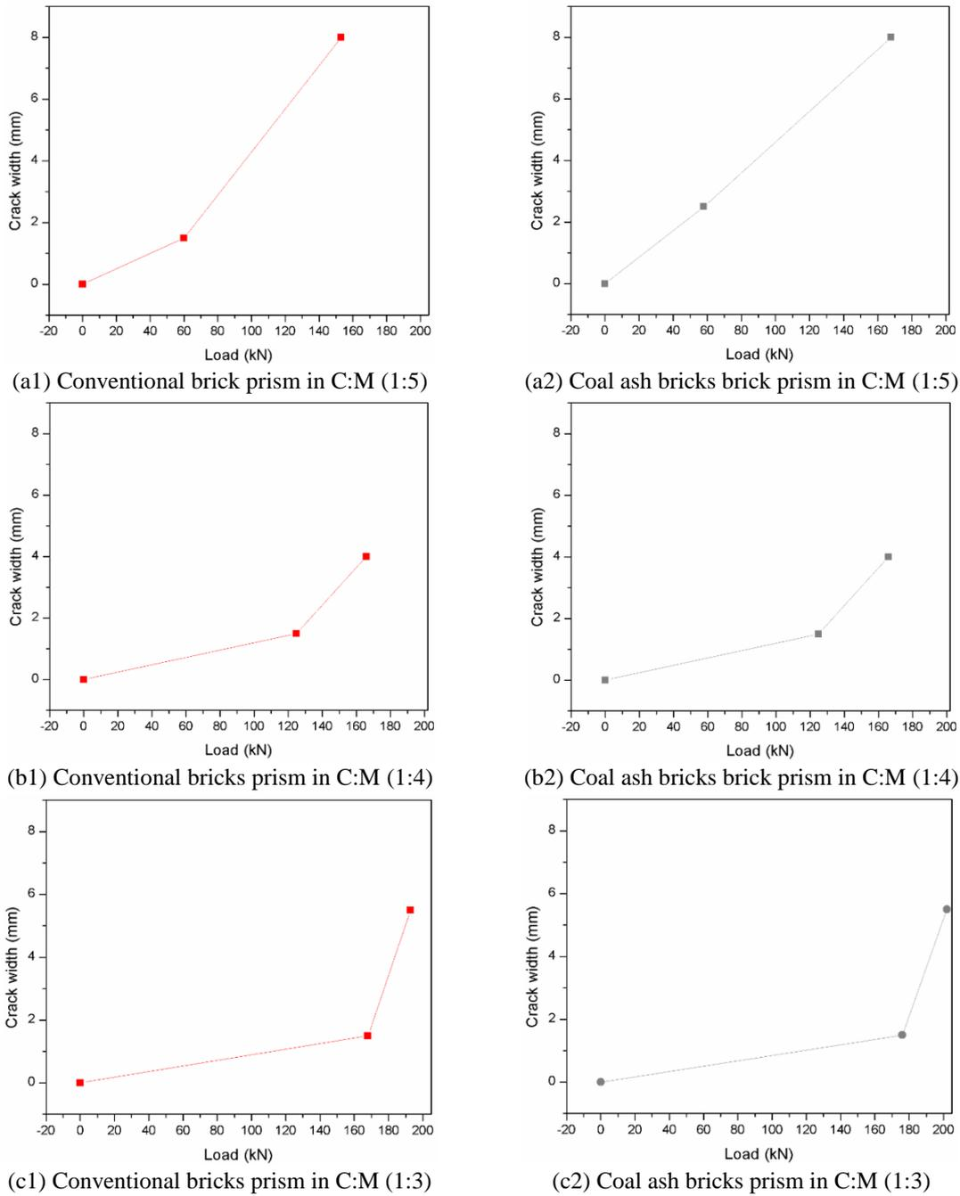
Fig. 7 Relationships between crack width and load applied for bricks
