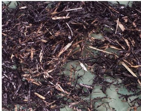
Fig. 4 Straws treated with bitumen
