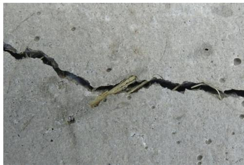
Fig. 8 Crack in the sample with straw after rupture
