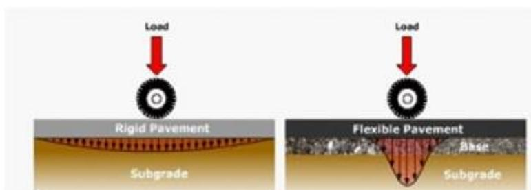
Fig. 2 Deflection of rigid and flexible pavement
